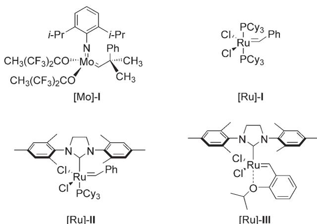
**Figure 1.** Commonly used metathesis catalysts.
