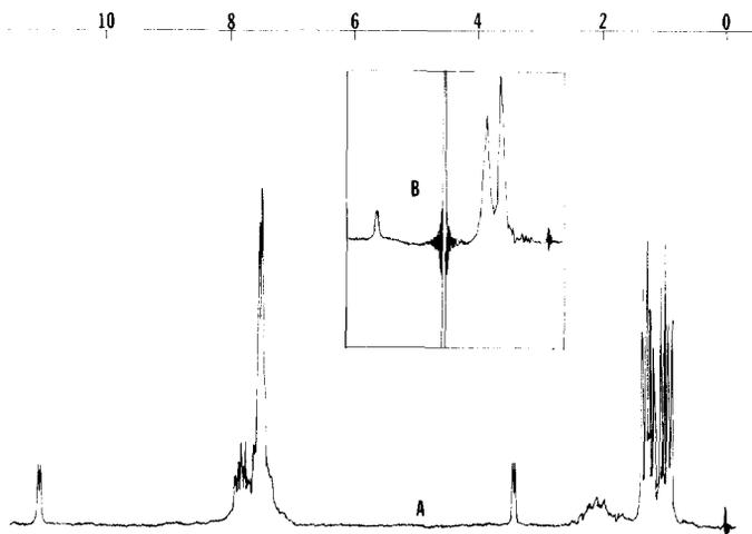
Fig. 4. Proton spectrum (1000 Hz) of  $\text{Ph}(i\text{-Pr})\text{P}(\text{O})\text{H}$  in  $\text{CDCl}_3$ . Spectrum A is the complete spectrum with the assignments given in Table 4. Spectrum B shows the collapse of the eight-line methyl resonance by double irradiation at the methine proton resonance.
