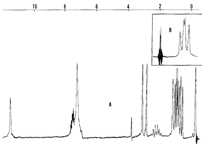
Fig. 6. Proton spectrum (1000 Hz) of  $\text{Ph}(i\text{-Pr})\text{P}(\text{O})\text{CH}_2\text{COOH}$  in  $\text{CDCl}_3$ . Spectrum A is the complete spectrum with assignments given in Table 6. Spectrum B shows the methyl region of the isopropyl group with double irradiation at the methine proton.
