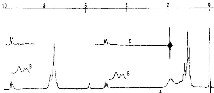
Fig. 5. Proton spectrum (1000 Hz) of  $Ph(sec-Bu)P(O)H$  in  $CDCl_3$ . Spectrum A is the complete spectrum. Spectrum B is an expanded view of the resonance due to the phosphorus proton. Spectrum C shows the phosphorus hydrogen region during double irradiation at the methine proton resonance.
