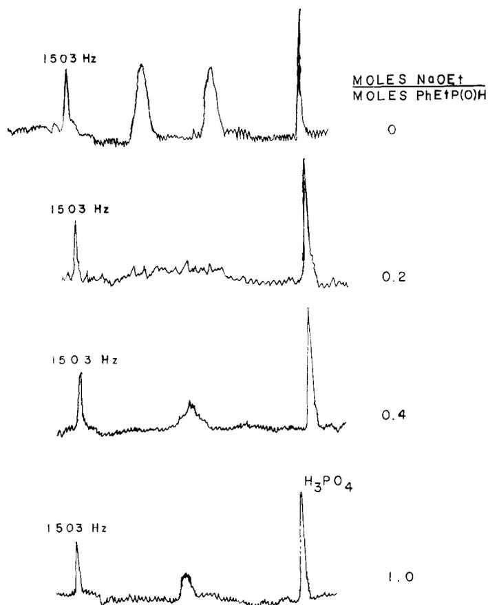
Fig. 1.  $^{31}\text{P}$  NMR spectra of  $\text{PhEtP}(\text{O})\text{H}$  upon addition of  $\text{NaOEt}$ .
