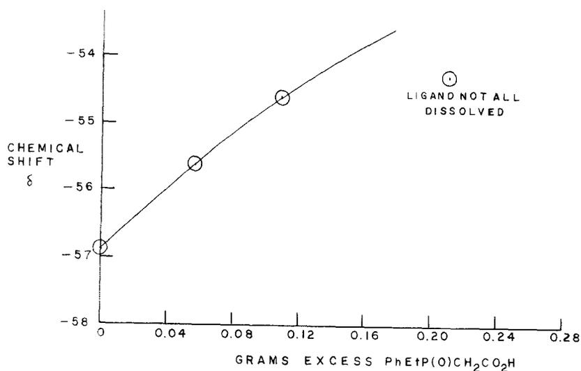
Fig. 7. The variation of the  $^{31}\text{P}$  chemical shift of  $[\text{PhEtP}(\text{O})\text{CH}_2\text{CO}_2]_2\text{UO}_2$  in  $\text{CH}_2\text{Cl}_2$  with excess phosphorylacetate ligand.
