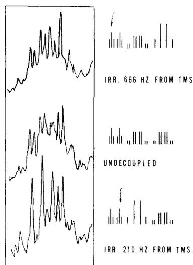
Fig. 3. Proton spectrum of the methylene region only (1.6–2.2  $\delta$ ) of  $\text{PhEtP}(\text{O})\text{H}$  (middle, undecoupled); with spin tickling of the low field PH triplet (upper spectrum); with spin tickling of the high field PH triplet (lower spectrum).
