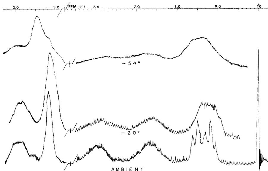
Fig. 8. Variable temperature proton spectra of  $[\text{PhEtP}(\text{O})\text{CH}_2\text{CO}_2]\text{UO}_2$  in  $\text{CDCl}_3$ .
