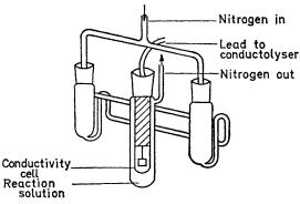
Conductivity apparatus for ' fast ' hydrolysis reactions
