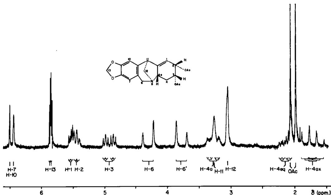
Fig. 1. 100 MHz NMR spectrum of diacetylbrunsvigine in  $\text{CDCl}_3$ .
