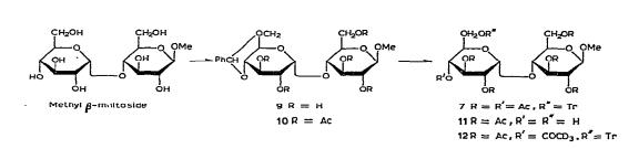
In an unambiguous synthesis of 7, methyl  $\beta$ -maltoside<sup>8</sup> was converted into the 4',6'-O-benzylidene acetal (9), which was acetylated to yield compound 10. Treatment with 50% acetic acid removed the benzylidene group to give compound 11, which upon tritylation followed by acetylation, gave compound 7.
