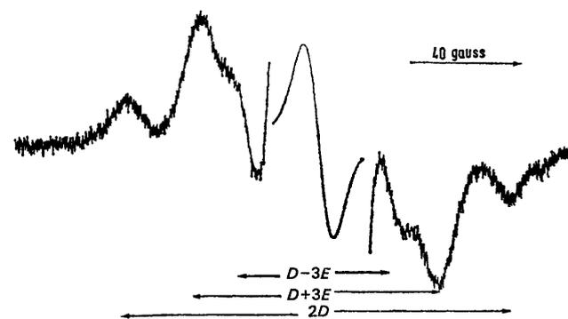
FIGURE 3 The electron resonance spectrum of a frozen solution of Schlenk's hydrocarbon (III) in toluene at 173 K
