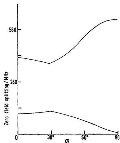
FIGURE 4 The zero-field splitting parameters  $D$  and  $E$  calculated for structure (III) as a function of the deviation from planarity
