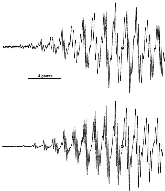
FIGURE 1 The solution electron resonance spectrum of radical (V). Only one half the spectrum is shown; the centre is marked by a circle. The upper spectrum is experimental and the lower is a simulation based on the coupling constants given in the Table
