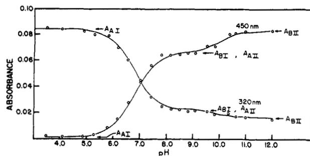
FIGURE 9: Spectrophotometric titration curves for 12.9  $\mu\text{M}$  papain-R at 320 and 450 nm. Solid lines are calculated titration curves for two acidic groups,  $pK_{I} = 6.79$ ,  $pK_{II} = 10$ , with  $A_{AI} = 0.084$ ,  $A_{BI} = A_{AII} = 0.022$ , and  $A_{BII} = 0.016$  at 320 nm, and  $A_{AI} = 0.001$ ,  $A_{BI} = A_{AII} = 0.066$ , and  $A_{BII} = 0.083$  at 450 nm.
