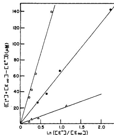
FIGURE 1: Determination of the ratio  $(k_1 + k_2^0)/k_3$ , pH 5.63; ( $\Delta$ ) pH 6.52, ( $\bullet$ ) pH 7.20, ( $\circ$ ) in 4.05 mM L-cysteine, 0.405 mM EDTA,  $\Gamma/2 = 0.12$ , 10% ethanol, 25°,  $[E^0] = 9\text{--}18 \mu\text{M}$ .
