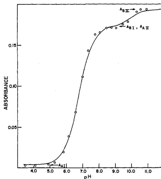
FIGURE 8: Spectrophotometric titration curve for  $12.9 \mu\text{M}$  papain-R at 410 nm. Conditions were the same as in Figure 7. Solid line is a calculated titration curve for two acidic groups  $pK_I = 6.79$ ,  $pK_{II} = 10$ . With  $A_{AI} = 0.003$ ,  $A_{BI} = A_{AII} = 0.173$ , and  $A_{BII} = 0.194$ .
