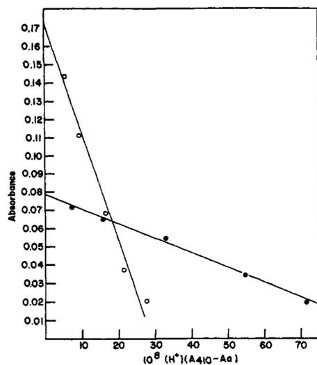
FIGURE 5: Determination of the ionization constant of the reporter group in **2** at  $5.00 \mu\text{M}$  **2**: (●) and in papain-R at  $12.9 \mu\text{M}$  papain-R; (○) using eq 10.  $A_A$  was set at 0.0018 and 0.0030 for **2** and papain-R, respectively.
