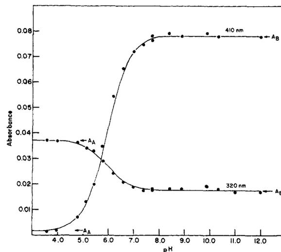
FIGURE 4: Spectrophotometric titration of  $5.00 \mu\text{M} **2** at 320 and 410 nm. Conditions were the same as in Figure 3. Solid lines calculated from eq 10 with  $K = 10^{-5.92}$ ,  $A_A = 0.0018$  and  $A_B = 0.0784$  at 410 nm, and  $A_A = 0.0370$  and  $A_B = 0.0176$  at 320 nm.$
