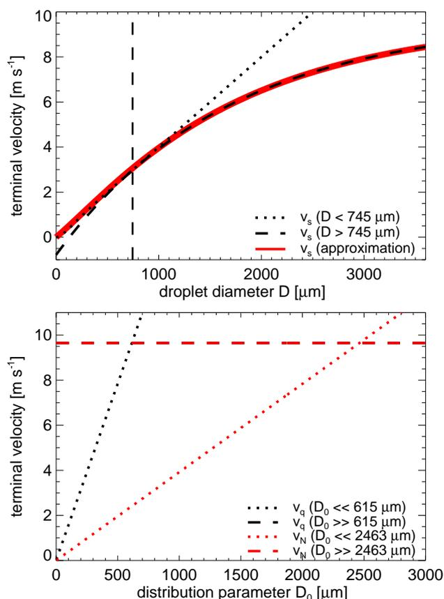
**Fig. 1.** Terminal velocity: The terminal velocity after Rogers et al. (1993) for small and large drops with the approximation for the whole size range (Eq. (11)=red curve) (upper panel); the fall velocity for the bulk mass and the bulk number concentration (Eq. (12)) (lower panel)
