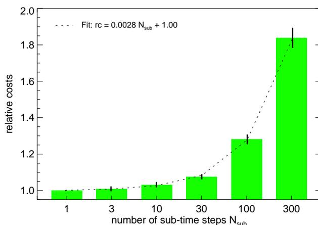
**Fig. 2.** Relative CPU time of simulations with different number of sub-time step compared to a simulation with one sub-time step. The vertical error bars denote the standard deviation and the dotted line represent the linear fit.
