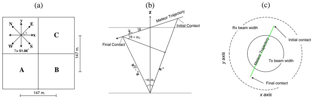
**Fig. 2.** (a) Antenna configuration for interferometric observations of meteors, note that the  $x$ -axis is rotated with respect to the East-West baseline  $\sim 51.06^\circ$ . Simplified geometry of a meteor trajectory respect to the illuminated beam: (b) altitudinal and (c) horizontal views.
