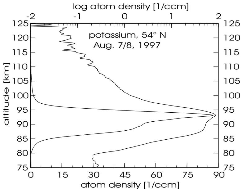
**Fig. 1.** K-layer of Aug. 7/8, 1997, 54° N on linear and logarithmic scales. The profile was obtained during 5 hours of integration. The sensitivity of the lidar allows it to detect free metal atoms at altitudes as high as 125 km altitude with densities as low as 0.05 atoms/cm<sup>3</sup>.
