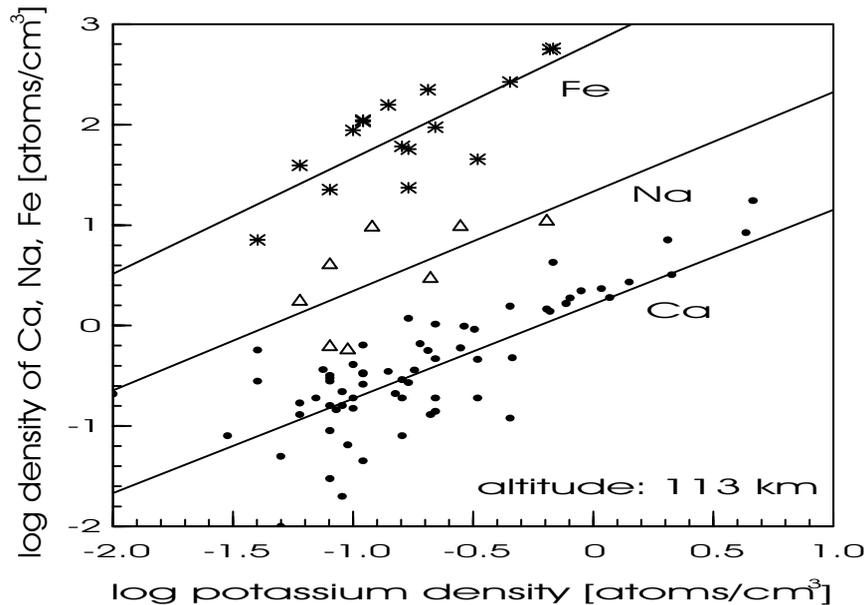
**Fig. 4.** Shown on a log-log plot are K densities versus Ca, Fe and Na at 113 km altitude from simultaneous observations at 54° N. All regressions have slopes close to one, which implies constant abundance ratios between all elements.
