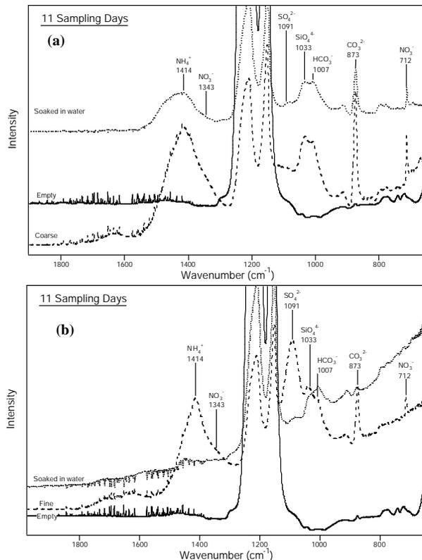
**Fig. 3.** FTIR-ATR spectra showing the inorganic ion bands for particles collected on Teflon filters during 11 consecutive sampling days. **(a)** shows the coarse particulate matters before and after soaking the filters in water and **(b)** shows fine particulate matters before and after soaking the filters in water for 24 h.
