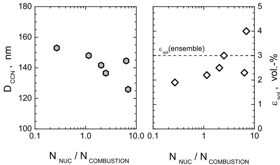
**Fig. 12.** Left panel: CCN activation diameter  $D_{CCN}$  plotted as a function of the ratio of nucleated particles  $N_{NUC}$  of size  $D < 10$  nm to combustion particles  $N_{COMBUSTION}$  of size  $D \geq 20$  nm for the high fuel sulphur case. Right panel: volume fraction of soluble matter calculated from the measured  $D_{CCN}$  values using Köhler theory (Eq. 3); the dashed line represents the ensemble value  $\epsilon_{sol}$  determined by the Köhler curve fitting all measurements.
