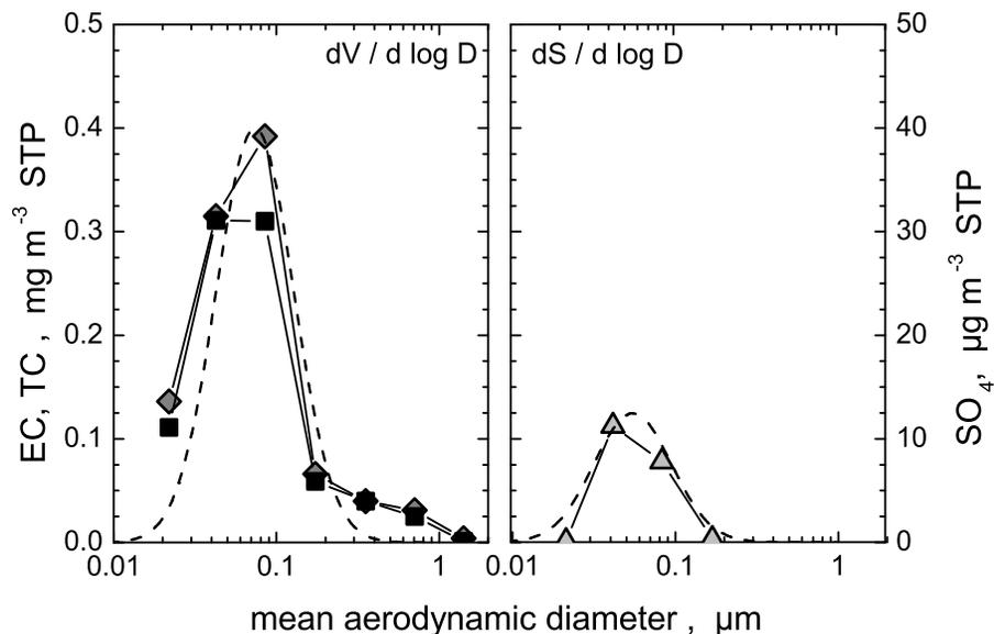
**Fig. 7.** Size-resolved chemical composition of combustor exhaust particles for high FSC fuel used; left panel shows the mass distribution of total (grey) and elemental (black) carbon together with a volume distribution calculated from measured size DMA spectra; right panel shows the mass distribution of sulphate together with a surface distribution calculated from measured spectra.
