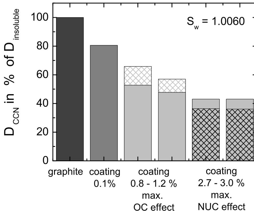
**Fig. 15.** Relative contribution of particle coating with sulphuric acid to the change in the CCN activation diameter of an initially insoluble graphite particle; the shaded bars represent the increase in  $D_{CCN}$  and thus the reduction in CCN activation by a large fraction of non-volatile OC (OC effect) and the further decrease in  $D_{CCN}$  and thus the enhancement of CCN activation by particle nucleation-coagulation (NUC effect).
