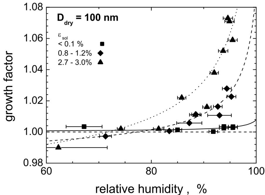
**Fig. 10.** Humidity growth of particles of initial size  $D_{dry}=100 \text{ nm}$  as a function of relative humidity for low, medium and high fuel sulphur cases; lines represent growth curves determined from Köhler theory for the indicated volume fractions of soluble matter  $\epsilon_{sol}$ .
