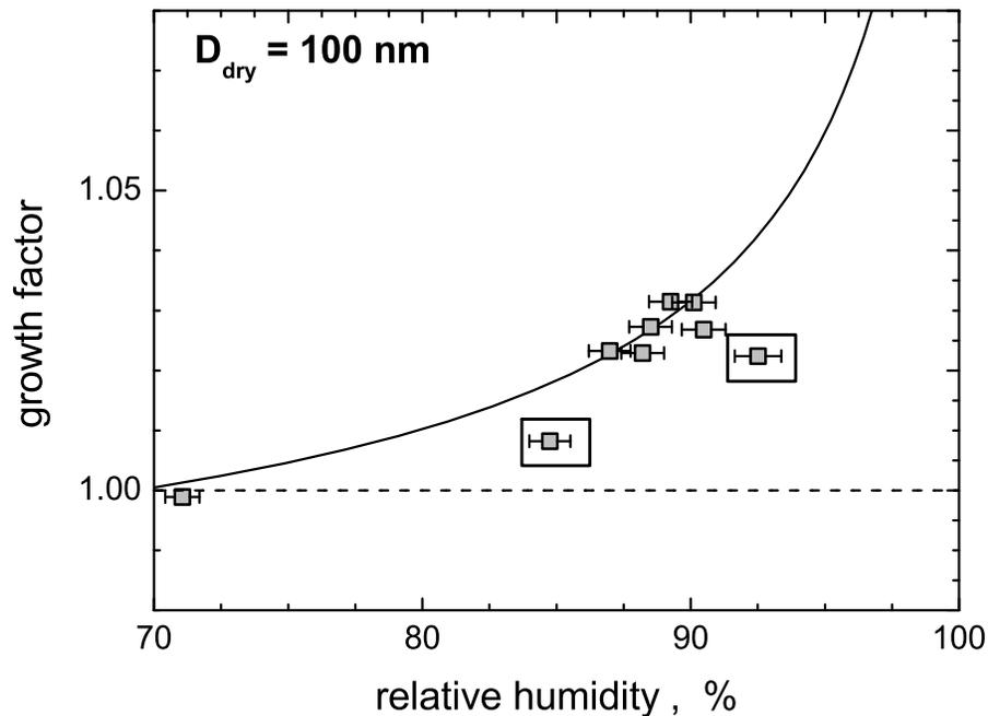
**Fig. 13.** Humidity growth of particles of initial size  $D_0=100$  nm as a function of relative humidity for the high fuel sulphur case; the indicated data points correspond to sampling points at the edge positions of the combustor exit nozzle plane.
