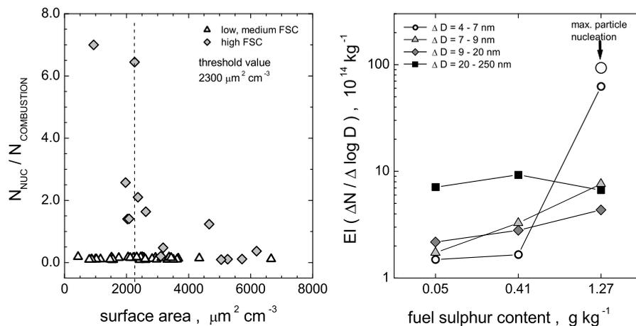
**Fig. 9.** Left: ratio of nucleated particles  $N_{NUC}$  of size  $D < 10 \text{ nm}$  to combustion particles  $N_{COMBUSTION}$  of size  $D \geq 20 \text{ nm}$  as a function of the surface area of the pre-existing combustion aerosol; the dashed line denotes the threshold value for particle nucleation of  $2300 \mu\text{m}^2 \text{cm}^{-3}$ . Right: number of particles per kg of consumed fuel in denoted diameter bins as a function of the fuel sulphur content.
