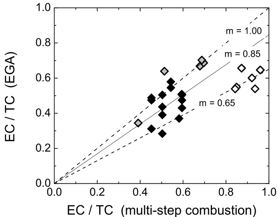
**Fig. 2.** Correlation of the ratio of elemental carbon to total carbon EC/TC as determined from evolved gas analysis EGA and multi-step combustion as a reference method; symbols represent data for low (open), medium (filled) and high (shaded) fuel sulphur content.
