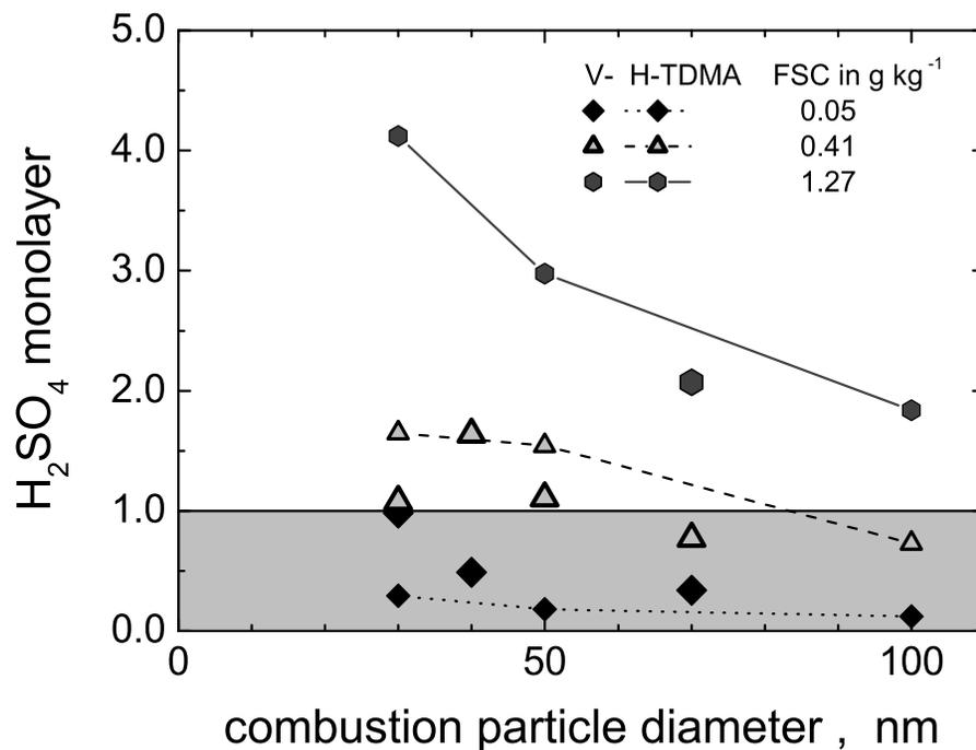
**Fig. 8.** Coverage of carbonaceous combustion particles in terms of monolayers of H<sub>2</sub>SO<sub>4</sub> for different levels of fuel sulphur content FSC; the coating was determined from measurements using Volatility Tandem DMA and Hygroscopicity Tandem DMA methods.
