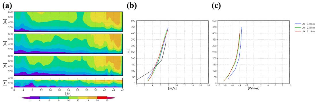
**Fig. 5.** Vertical profiles of **(a)** horizontal wind speed [m/s] as 48h time series at Kivenlathi mast for LM 7.0 km, 2.8 km, 1.1 km grid resolution and observations (top to bottom), **(b)** wind speed [m/s] for 28 December 1995, +6 h, **(c)** potential temperature [°C] for 28 December 1995, 00:00 UTC+6 h.
