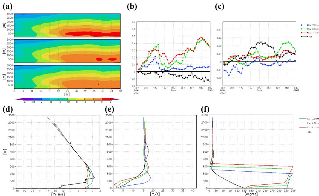
**Fig. 11.** LM simulations with 7, 2.8 and 1.1 km resolution on 6 January 2003, **(a)** Blindern, time series of vertical temperature [°C], 48 h forecast starting 00:00 UTC+00 h. Time series of vertical temperature gradient [°C/m] for **(b)** Hovin and **(c)** Tryvann/Blindern. Forecasts for 6 January 2003, 00:00 UTC+24 h, vertical LM profiles and radiosoundings at Blindern for **(d)** temperature [°C], **(e)** horizontal wind speed [m/s], **(f)** horizontal wind direction [°].
