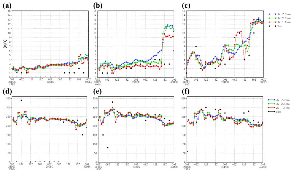
**Fig. 6.** Time series of 10 m horizontal winds for 48 h LM forecasts for 7.0 km, 2.8 km, 1.1 km resolution starting 28 December 1995, 00:00 UTC, top: wind speed [m/s] for (a) Vantaa, (b) Kaisaniemi, (c) Isosaari, and bottom: wind direction for (d) Vantaa, (e) Kaisaniemi, (f) Isosaari.
