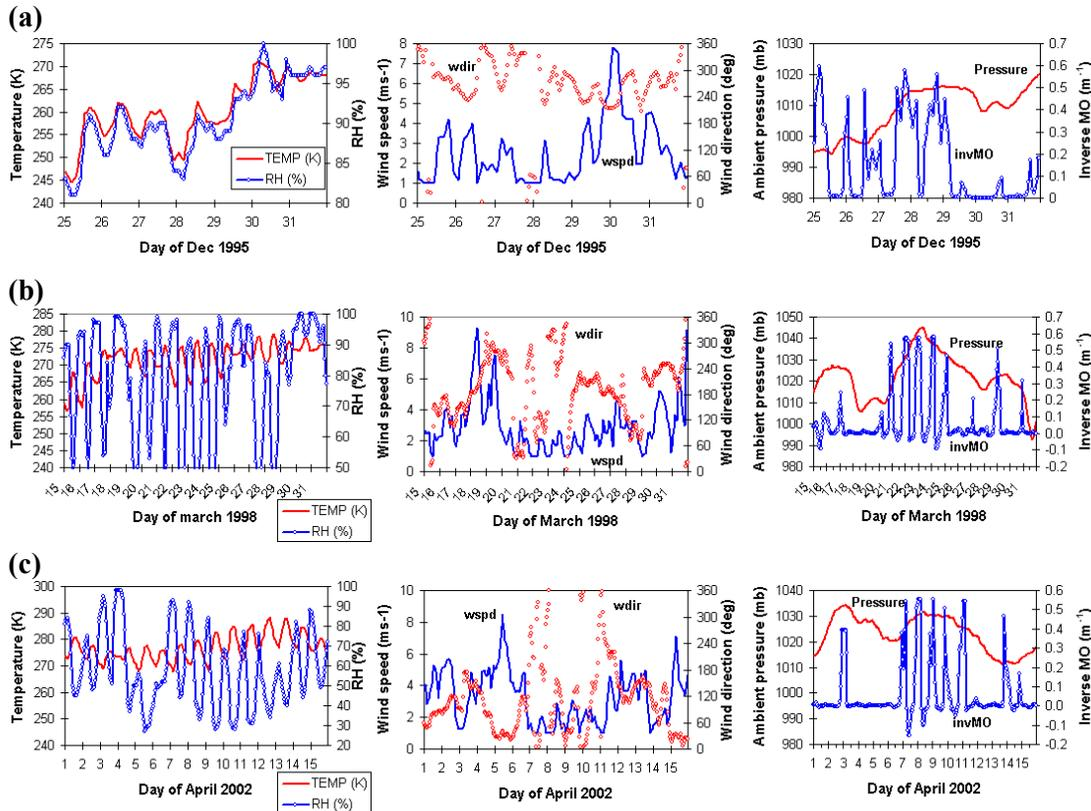
**Fig. 2.** Meteorological observations (plus FMI-MPP-model-derived inverse Monin-Obukhov number stability index) at Helsinki-Vantaa airport for **(a)** December 1995, **(b)** March 1998, **(c)** April 2002 (from FUMAPEX data web pages of the Finnish Meteorological Institute).
