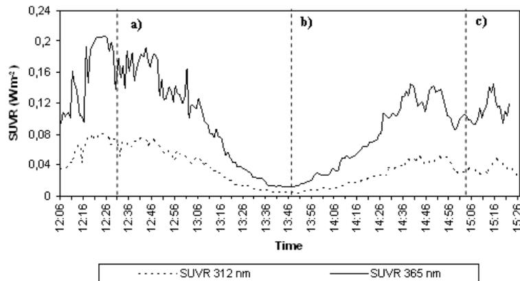
**Fig. 4.** SUVR (312 and 365 nm) measurements derived from the VLX-3W radiometer (Vilber-Lourmat, France), before, during and after the solar eclipse of 29 March 2006, at Athens, **(a)** beginning of the solar eclipse, **(b)** solar eclipse maximum, **(c)** end of the solar eclipse.
