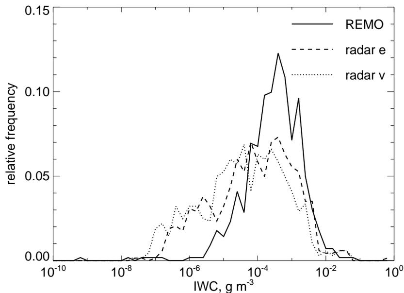
**Fig. 24.** Probability density functions of IWC derived from REMO and from cloud radar (using the algorithm of Hogan et al., 2006) in the range of 6000 m to 10 000 m. The abbreviations “e” and “v” stand for the  $Z$ -IWC – algorithms optimizing the expected value and the variance of IWC, respectively.
