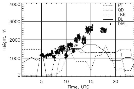
**Fig. 17.** ABL height derived from REMO and from DIAL on 10 June 2003 (top) and 7 June 2004 (bottom). The model ABL height is derived from the gradient of potential temperature (PT), of specific humidity (QD), of turbulent kinetic energy (TKE) and from static stability (BL, see chapter 2).
