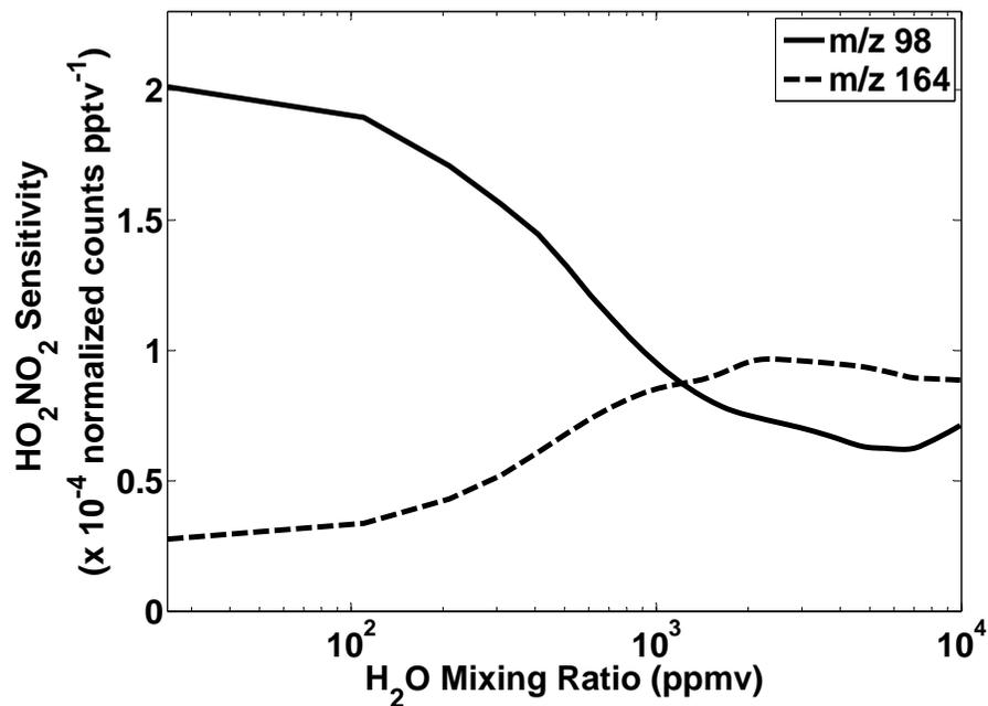
**Fig. 1.** Sensitivity curves for  $m/z$  98 (solid) and  $m/z$  164 (dash) as a function of  $\text{H}_2\text{O}$  mixing ratio in the flow tube. The sensitivity curves are used to calculate the final mixing ratios of  $\text{HO}_2\text{NO}_2$ .
