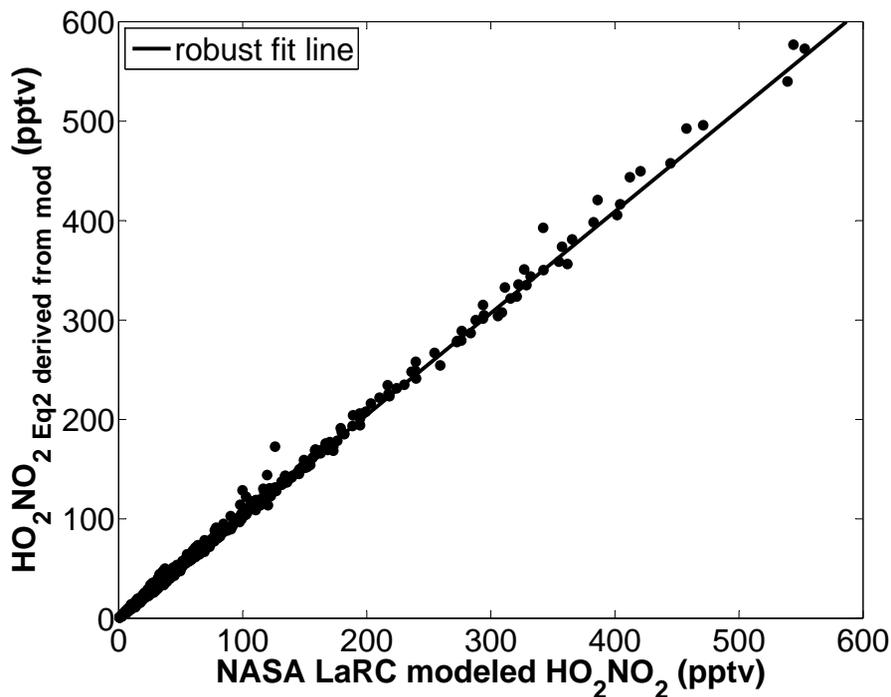
**Fig. 3.**  $[\text{HO}_2\text{NO}_2]_{\text{SS}}$ , calculated from Eq. (2), using modeled values of  $\text{HO}_2$  and  $\text{NO}_2$  versus  $\text{HO}_2\text{NO}_2$  predicted by the NASA LaRC box model. The slope of the robust fit line is 1.02; intercept is 0.10 pptv;  $R^2=0.99$ , demonstrating that Eq. (2) is a valid simplification under MILAGRO conditions.
