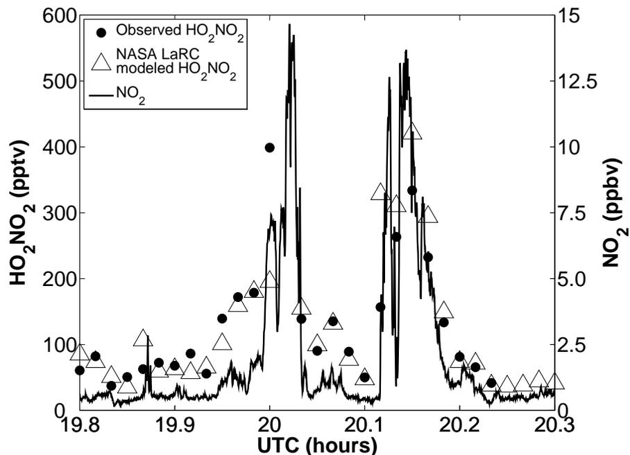
**Fig. 4.** Mixing ratios of  $\text{HO}_2\text{NO}_2$  and  $\text{NO}_2$  during Flight 29 March 2006 in an air mass heavily impacted by pollution. Dots are CIMS measurements of  $\text{HO}_2\text{NO}_2$ . Triangles are NASA LaRC box model values of  $\text{HO}_2\text{NO}_2$ . The solid line is observed  $\text{NO}_2$  mixing ratio. Variations in the observed and modeled  $\text{HO}_2\text{NO}_2$  mixing ratios closely follow variations in  $\text{NO}_2$ .
