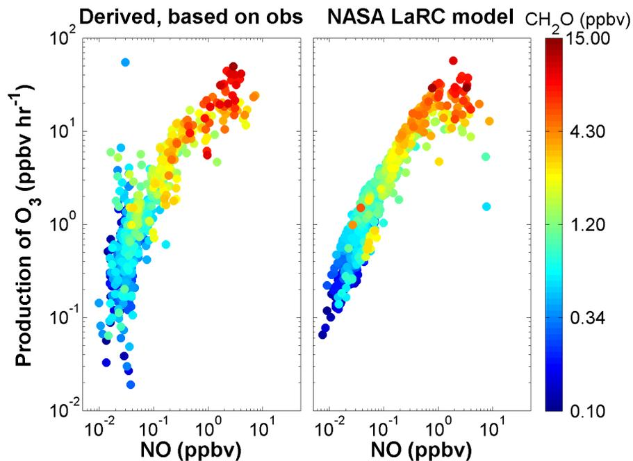
**Fig. 8.** Rate of ozone production versus mixing ratio of NO colored by the mixing ratio of formaldehyde.  $P_{O_3}$  derived from Eq. (6), based on measurements of  $HO_2NO_2$  and  $NO_x$  are shown in the left panel. NASA LaRC box model predictions of  $P_{O_3}$  are shown in the right panel.
