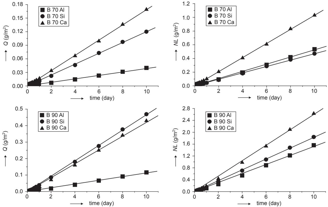
Figure 1. Time dependence of the amounts and normalized amounts of leached elements at temperatures 70°C a 90°C for leaching solution B. Lines represent the linear regression model.
