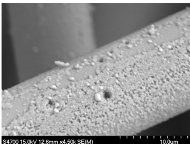
Figure 3. SEM micrographs of corroded fibers.
