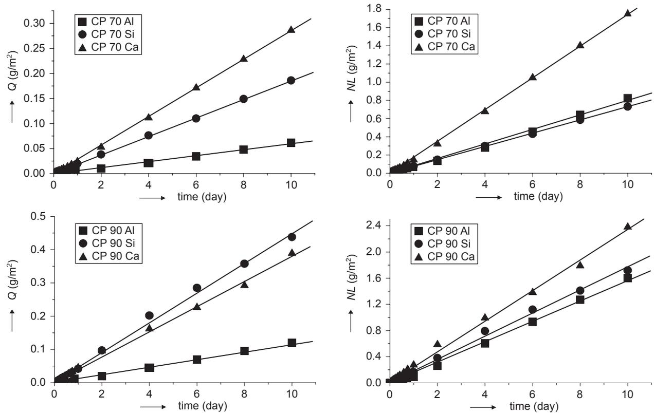
Figure 2. Time dependence of the amounts and normalized amounts of leached elements at temperatures 70°C a 90°C for leaching solution CP. Lines represent the linear regression model.
