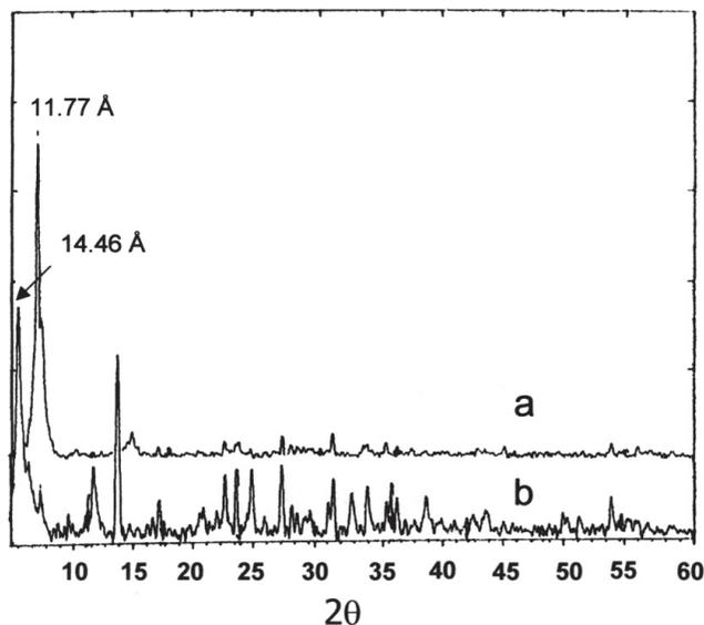
Fig. 3. Powder X-ray diffractions patterns of a)  $\text{Li}_{0.43}\text{K}_{0.57}\text{BiP}_2\text{S}_6$  b)  $\text{Li}_{0.43}(\text{PEO})_{2.4}(\text{H}_2\text{O})_{1.4}\text{K}_{0.57}\text{BiP}_2\text{S}_6$
