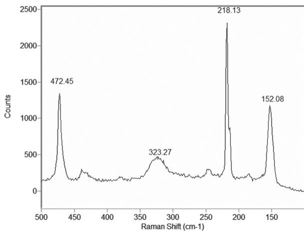
Fig. 2. Raman Spectra for  $\text{Li}_{0.38}\text{K}_{0.62}\text{SbP}_2\text{S}_6$
