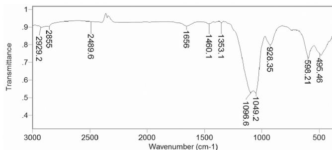
Fig. 4. FT-IR spectra for  $\text{Li}_{0.43}(\text{PEO})_{2.4}(\text{H}_2\text{O})_{1.4}\text{K}_{0.57}\text{BiP}_2\text{S}_6$
