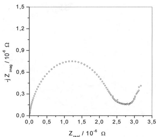
Fig. 5. Impedance plot and Nyquist diagram for  $\text{Li}_{0.43}(\text{PEO})_{2.4}(\text{H}_2\text{O})_{1.4}\text{K}_{0.57}\text{BiP}_2\text{S}_6$
