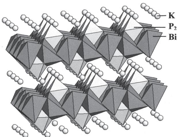
Fig. 1. Crystal structure of  $\text{KBi}_2\text{S}_6$  viewed along a-axis
