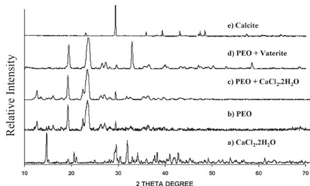
**Fig. 1.** X-ray powder diffraction patterns of a) calcium chloride starting material, b) a poly(ethylene oxide) film, c) a poly(ethylene oxide) and calcium chloride film, d)  $\text{CaCO}_3$  (vaterite) grown in a poly(ethylene oxide) film, e)  $\text{CaCO}_3$  (calcite) precipitated by exposure of a calcium chloride solution to a source of carbon dioxide.
