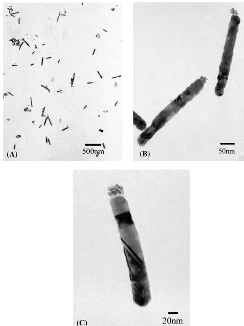
**Fig. 6** TEM images of nanostructure with nanoparticles/dithiols junction between gold segments nanowire
