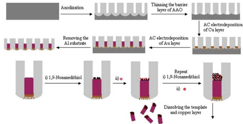
**Fig. 1** Schematic diagram describing the fabrication steps of nano “cigars” based on the porous AAO template. Prior to the electrodeposition step, the thinning of the barrier layer is necessary to form the dendrite structure at the bottom. The copper as the first layer was electrodeposited and gold is then
