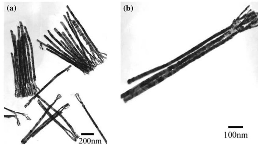
**Fig. 5** TEM images of gold nanorods functionalised by gold nanoparticles (A) the large scale of gold nanorods dispersed by aminodextran (B) two gold nanorods with the smooth bottom after removing the branch part of copper metal (C) the nanorod was selectively modified by gold nanoparticles, which look like the “lighting cigarette”
