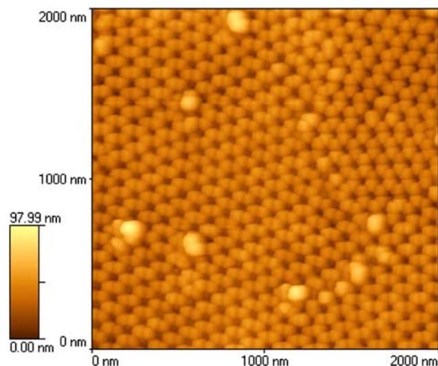
**Fig. 3** AFM top-view micrograph of the as-prepared AAO template by two-step anodization with the pore diameter of 40 nm
