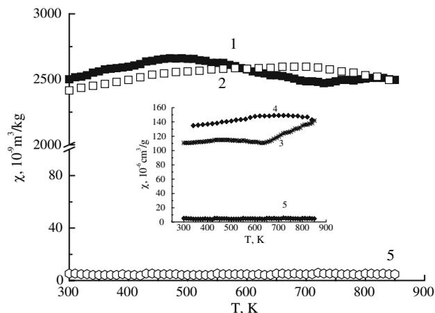
**Fig. 6**  $\chi(T)$  dependency for specimens #3 after different stages of thermochemical treatment: 1 and 2, #3 (heating and cooling, respectively); 5, #3-TC; inset: 3 and 4, #3-C (heating and cooling, respectively); 5, #3-TC
