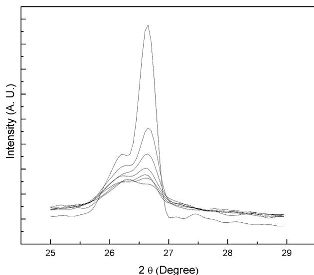
**Fig. 4** Variation in the quartz peak ( $2\theta = 26.58^\circ$ ) height and width with milling times
