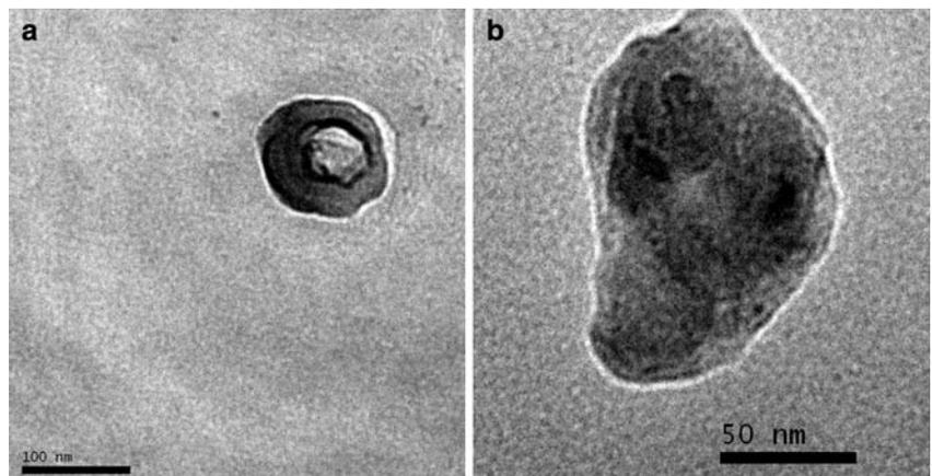
The characteristic –OH stretching vibration peak intensity increases by ball milling. The fly ash becomes more amorphous and the crystallite size reduces drastically. The shape and surface texture of the fly ash has been changed by ball milling which is evident from TEM and SEM studies. The nanostructured fly ash may be effectively used as reinforcing filler in polymer matrices.
