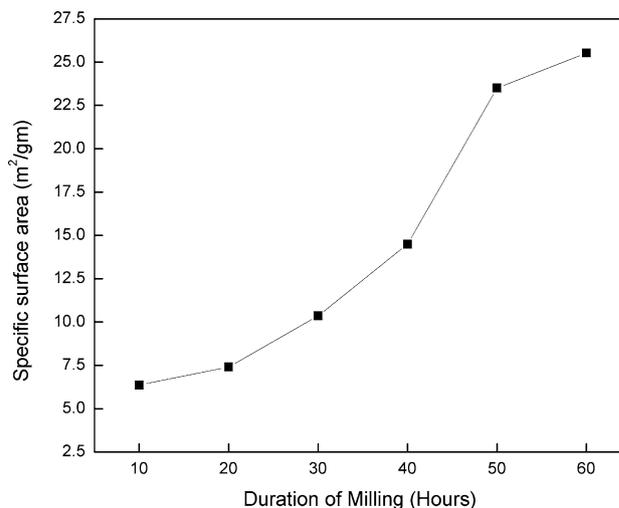
**Fig. 2** Variation of Specific surface area of fly ash with milling time (in hours)**Table 3** Surface energy and work of adhesion of fresh as well as ball milled fly ash
