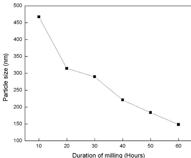
**Fig. 1** Variation in Particle size of fly ash with milling time (in hours)
