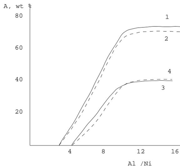
**Figure 1.** The influence of Al/Ni correlation on the conversion of propylene (A) on the catalytic system Ni-zeolite +  $\text{AlEt}_2\text{Cl}$  at 300 K ( $\text{Ni}^{2+}$  exchange degree-65%. 1) NiNaY; 2) NiNaX; 3) Ni-eryonite 4) Ni-mordenite.
