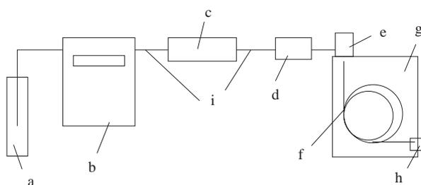
**Figure 2.** Schematic diagram of on-line SFE-SFC system a) CO<sub>2</sub> cylinder b) pump c) extraction vessel d) cryotrap-heater e) injection port f) chromatography column g) column oven h) detector i) transfer lines.
