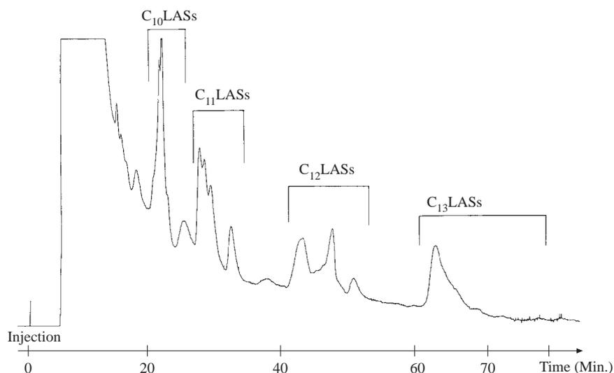
**Figure 6.** HPLC chromatogram of the LASs and SPCs isolated from Severn River sediment.
