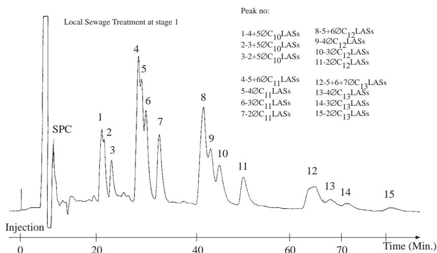
**Figure 4.** HPLC chromatogram of the LASs and SPCs isolated from local sewage treatment at stage 1.
