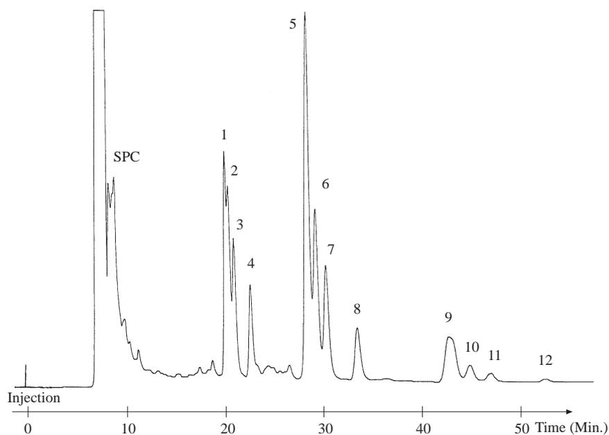
**Figure 5.** HPLC chromatogram of standard LASs and SPCs isolated from sediment.
