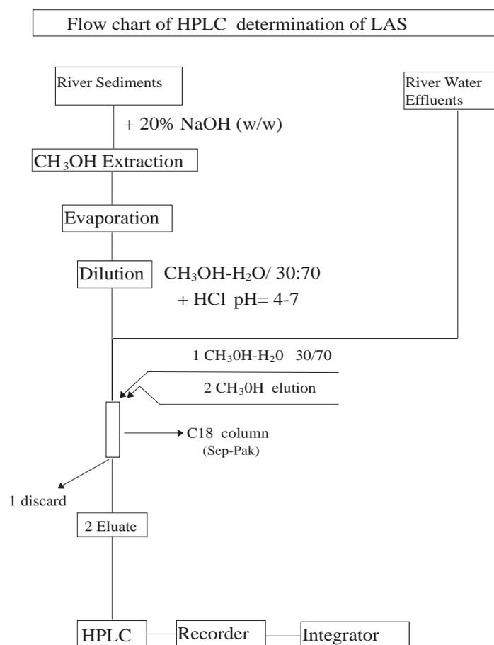
Figure 2. Flow chart of HPLC determination of LAS.
