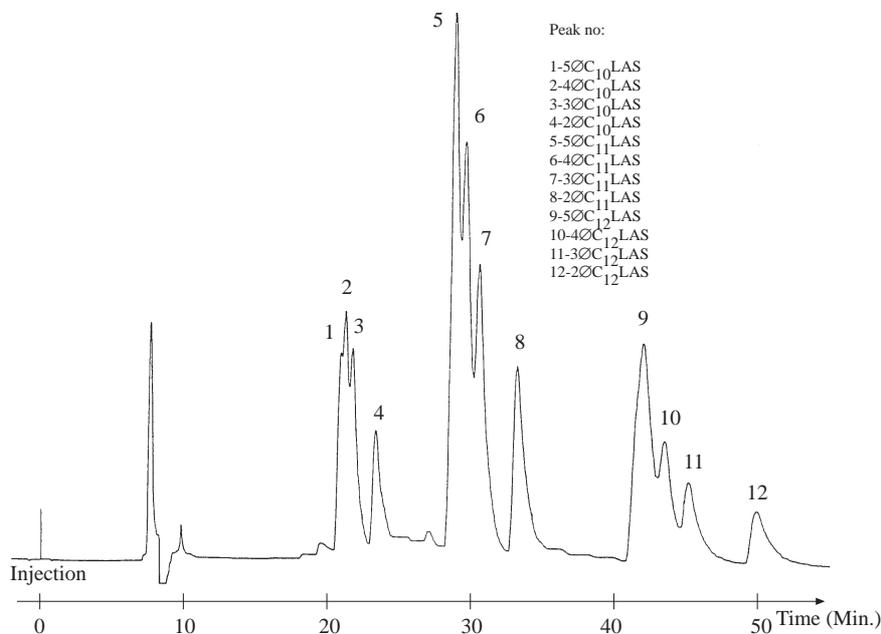
**Figure 3.** HPLC chromatogram of linear alkylbenzene sulphonic acid standards.
