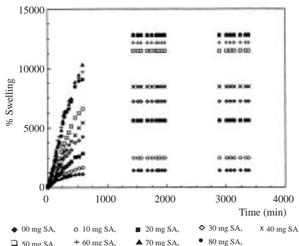
Figure 4. Swelling isotherms of AAm/SA hydrogels crosslinked by NBisA
