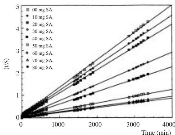
**Figure 6.** Swelling rate curves of AAm/SA hydrogels crosslinked by TMPTA.
