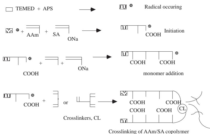
**Scheme 1.** Copolymerization and crosslinking mechanism of AAm/SA hydrogels.
