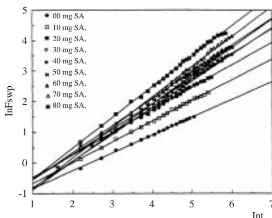
**Figure 7.** Swelling kinetics curves of AAm/SA hydrogels crosslinked by EGDMA.
