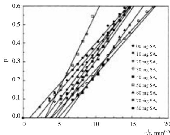
**Figure 8.** Diffusion curves of AAm / SA hydrogels crosslinked by BDMA.
