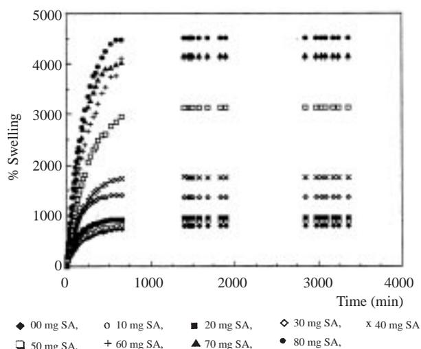
Figure 3. Swelling isotherms of AAm/SA hydrogels crosslinked by TMPTA
