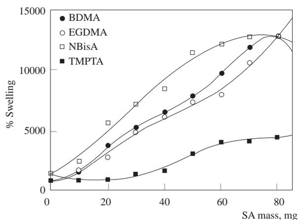
Figure 5. Effect of crosslinkers on swelling of AAm/SA hydrogels.
