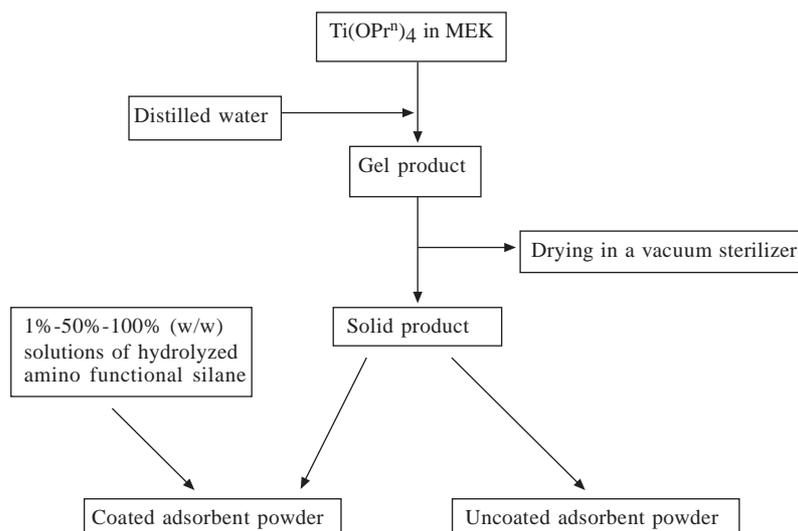
**Figure 1.** The procedure for the preparation of coated and uncoated adsorbent powders.
