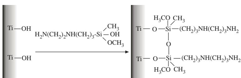
**Figure 2.** The bonding reaction between  $\text{TiO}_2$  surface and the coating material.
