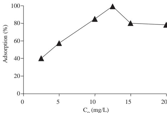
**Figure 3.** The effect of initial concentration on the adsorption percentages of  $\text{Fe}^{3+}$ .
