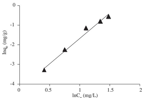
**Figure 4.** Freundlich isotherm for adsorption of  $\text{Fe}^{3+}$  on Amino-2 coated adsorbent.
