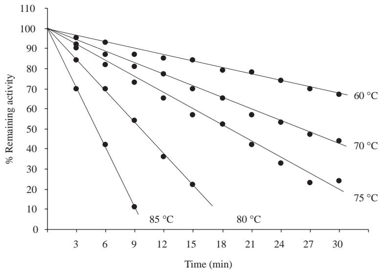
**Figure 2a.** Thermal inactivation of partially purified PPO at pH 7.2 in 10 mL 0.2 M phosphate buffer containing PPO enzyme.
