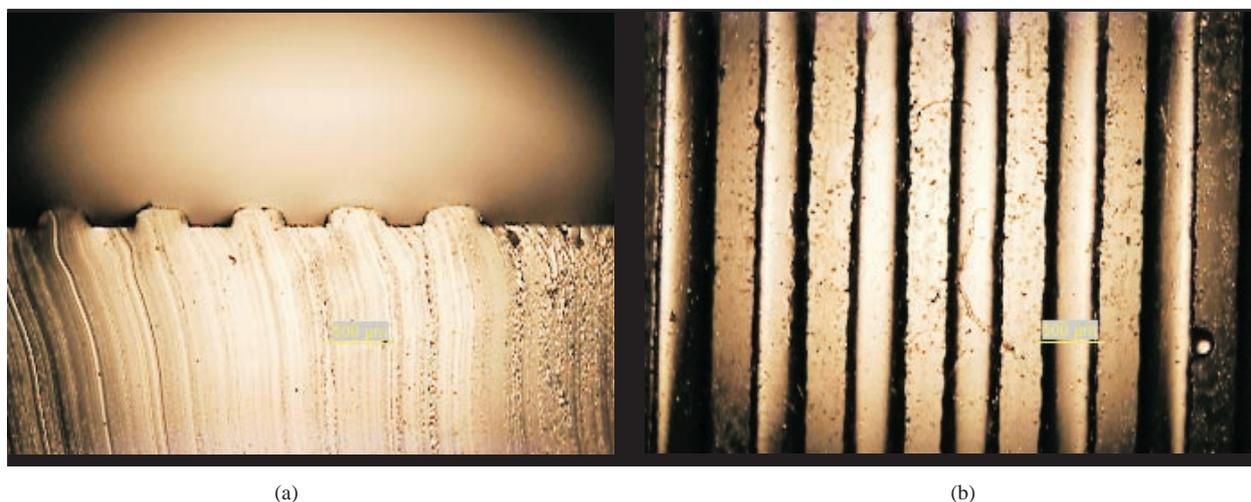
**Figure 1.** Optical microscopic images of the PDMS stamps. The bar represents 300  $\mu$ m. (a) cross-sectional view, (b) front view.
