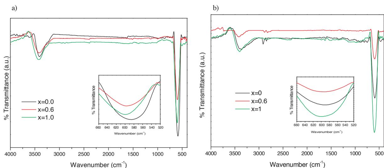
**Figure 3.** FTIR spectra of  $\text{Ni}_x\text{Co}_{1-x}\text{Fe}_2\text{O}_4$  NPs ( $x = 0.0, 0.6, 1.0$ ) hydrolyzed with: (a) NaOH and (b)  $\text{NH}_3$ .
