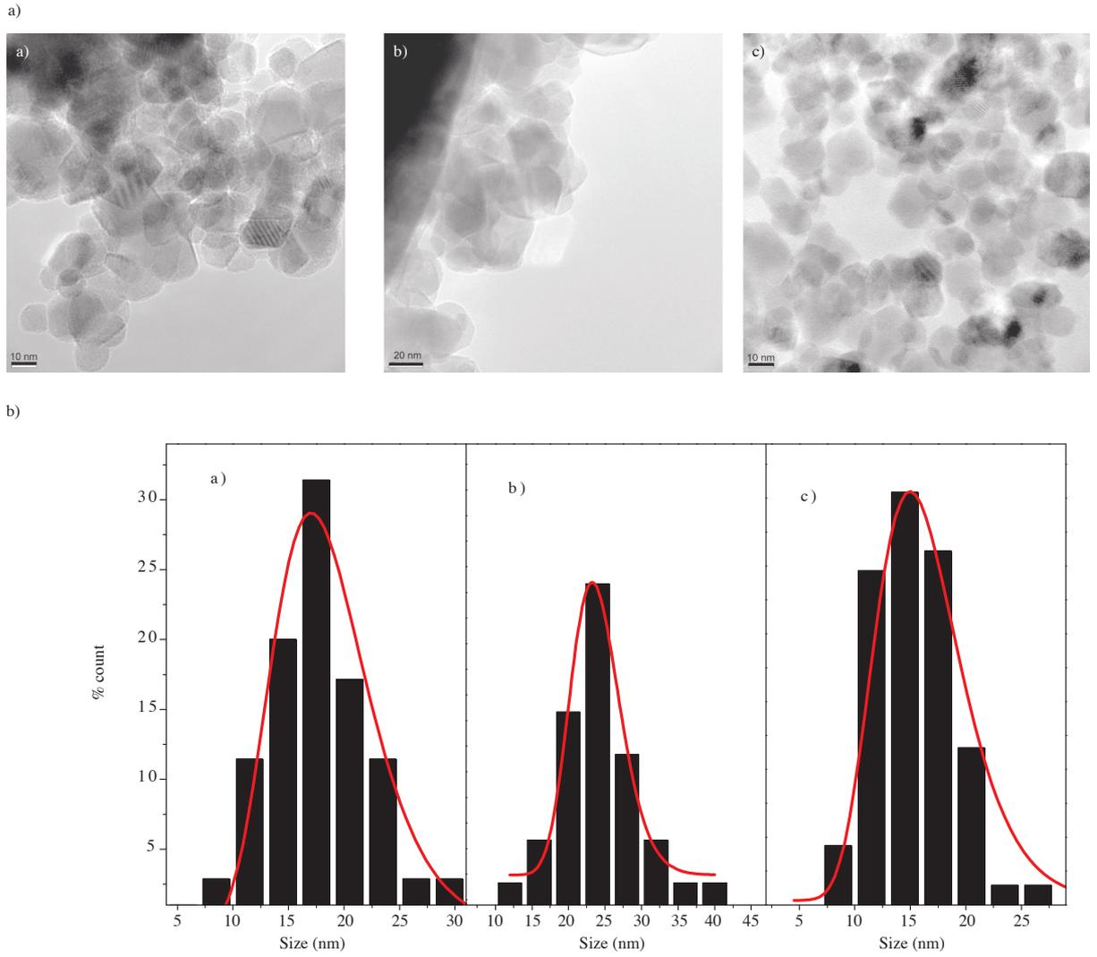
**Figure 5.** a) TEM micrographs of samples hydrolyzed by  $\text{NH}_3$  with the composition  $\text{Ni}_x\text{Co}_{1-x}\text{Fe}_2\text{O}_4$  where  $x$  is (a) 0.0, (b) 0.6, and (c) 1.0. b) Size distribution histograms and log normal fits for  $\text{Ni}_x\text{Co}_{1-x}\text{Fe}_2\text{O}_4$  NPs ( $x = 0.0, 0.6, 1.0$ ) hydrolyzed with  $\text{NH}_3$ .
