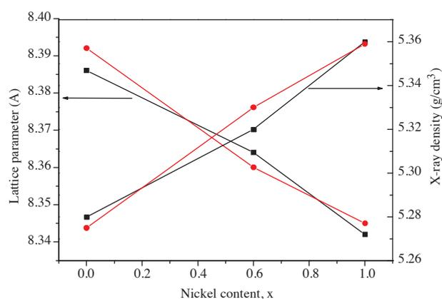
**Figure 2.** Variation of lattice parameter, and density of  $\text{Ni}_x\text{Co}_{1-x}\text{Fe}_2\text{O}_4$  NPs ( $x = 0.0, 0.6, 1.0$ ) (hydrolyzed with NaOH (red line) and  $\text{NH}_3$  (black line)) vs. nickel concentration.
