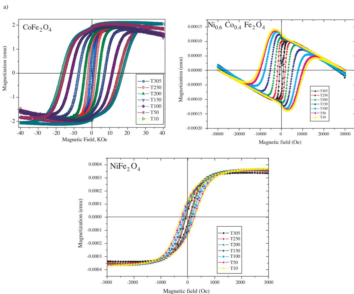
**Figure 6.** Magnetic hysteresis graphs of  $\text{Ni}_x\text{Co}_{1-x}\text{Fe}_2\text{O}_4$  NPs ( $x = 0.0, 0.6, 1.0$ ) hydrolyzed by a)  $\text{NaOH}$  b)  $\text{NH}_3$  at some selected temperatures.
