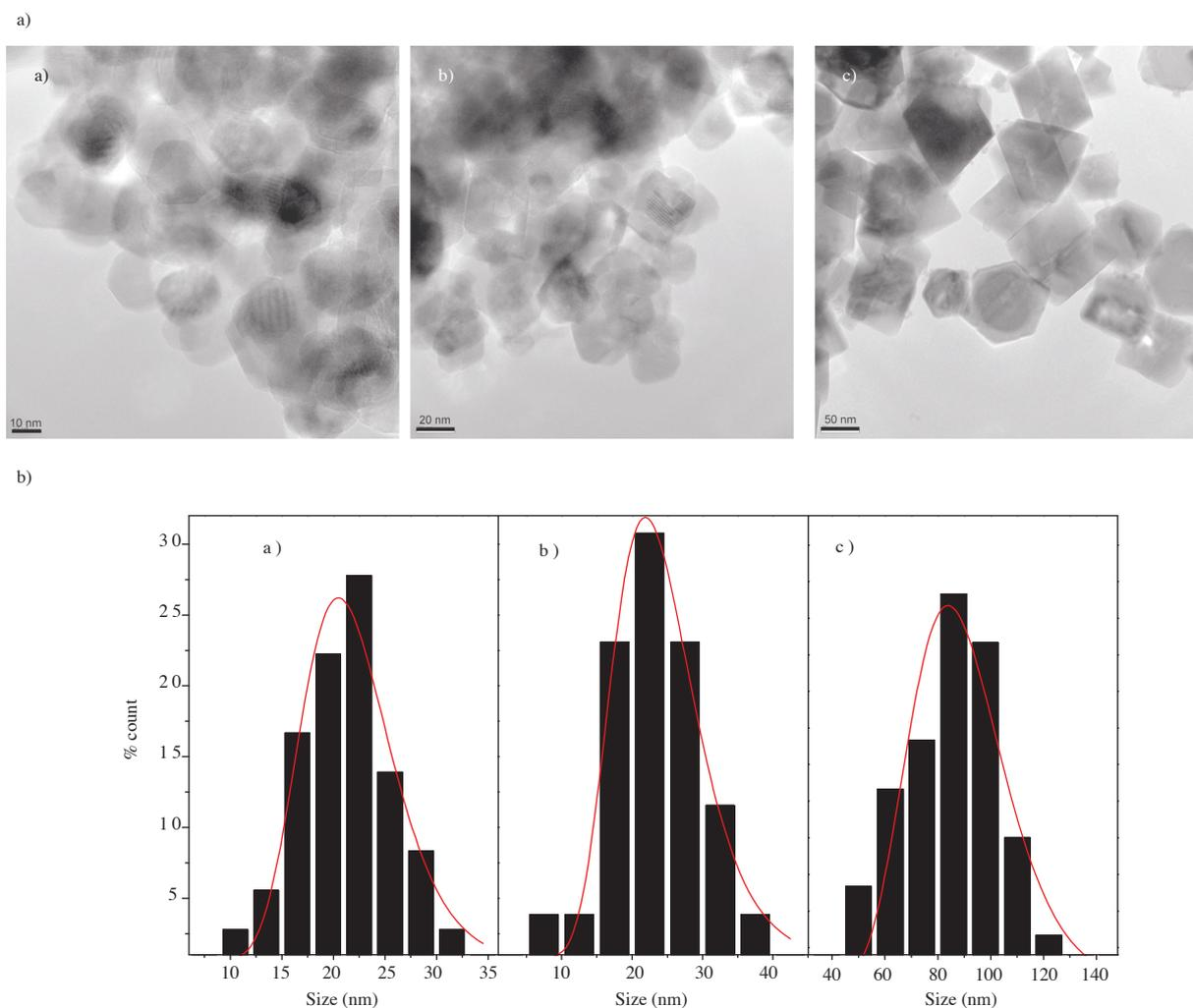
**Figure 4.** a) TEM micrographs of samples hydrolyzed by NaOH with the composition  $\text{Ni}_x \text{Co}_{1-x} \text{Fe}_2 \text{O}_4$  where  $x$  is (a) 0.0, (b) 0.6, and (c) 1.0. b) Size distribution histograms and log normal fits for  $\text{Ni}_x \text{Co}_{1-x} \text{Fe}_2 \text{O}_4$  NPs ( $x = 0, 0.6, 1$ ) hydrolyzed with NaOH.
