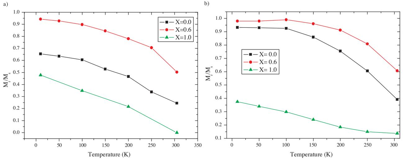
**Figure 8.** Mr/Ms curves for  $\text{Ni}_x\text{Co}_{1-x}\text{Fe}_2\text{O}_4$  NPs ( $x = 0.0, 0.6, 1.0$ ) hydrolyzed with: (a) NaOH and (b)  $\text{NH}_3$ .
