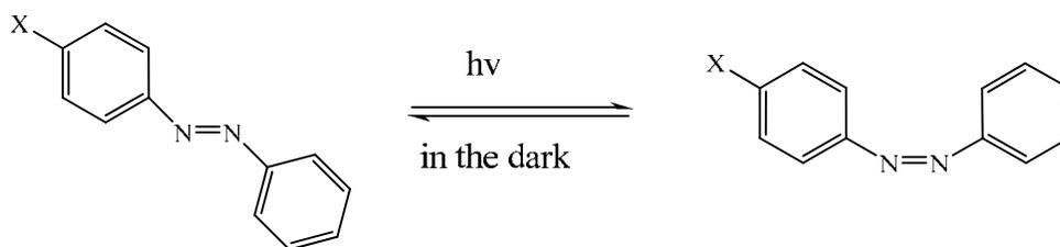
**Scheme 1.** *Z-E* interconversion of 4-*X*-azobenzenes (*X* = H, CH<sub>3</sub>, *n*-Butyl, OCH<sub>3</sub>, *O**t*-Butyl, Br, F, CF<sub>3</sub>).
