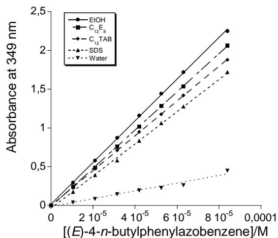
**Figure 1.** Lambert-Beer plot for (*E*) 4-*n*-Butyl azobenzene in ethanol, pure water,  $1 \times 10^{-2}$  M C<sub>12</sub>E<sub>8</sub>,  $2 \times 10^{-2}$  M C<sub>12</sub>TAB and  $2 \times 10^{-2}$  M SDS solutions.
