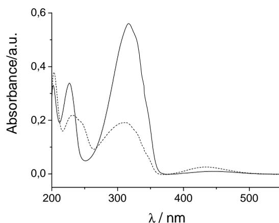
**Figure 2.** UV-vis spectra of azobenzene before (*E* isomer, solid line) and after (*Z* isomer, dotted line) UV irradiation.
