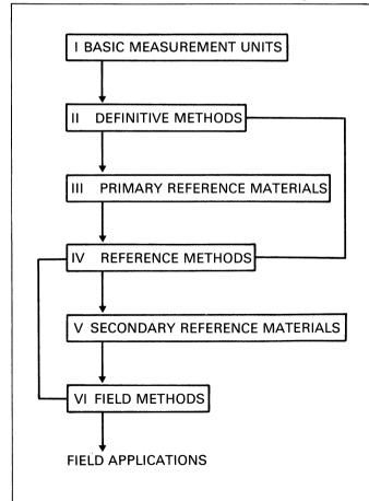
Figure 1. Six basic technical components of an idealised accuracy-based compatible measurement system.
