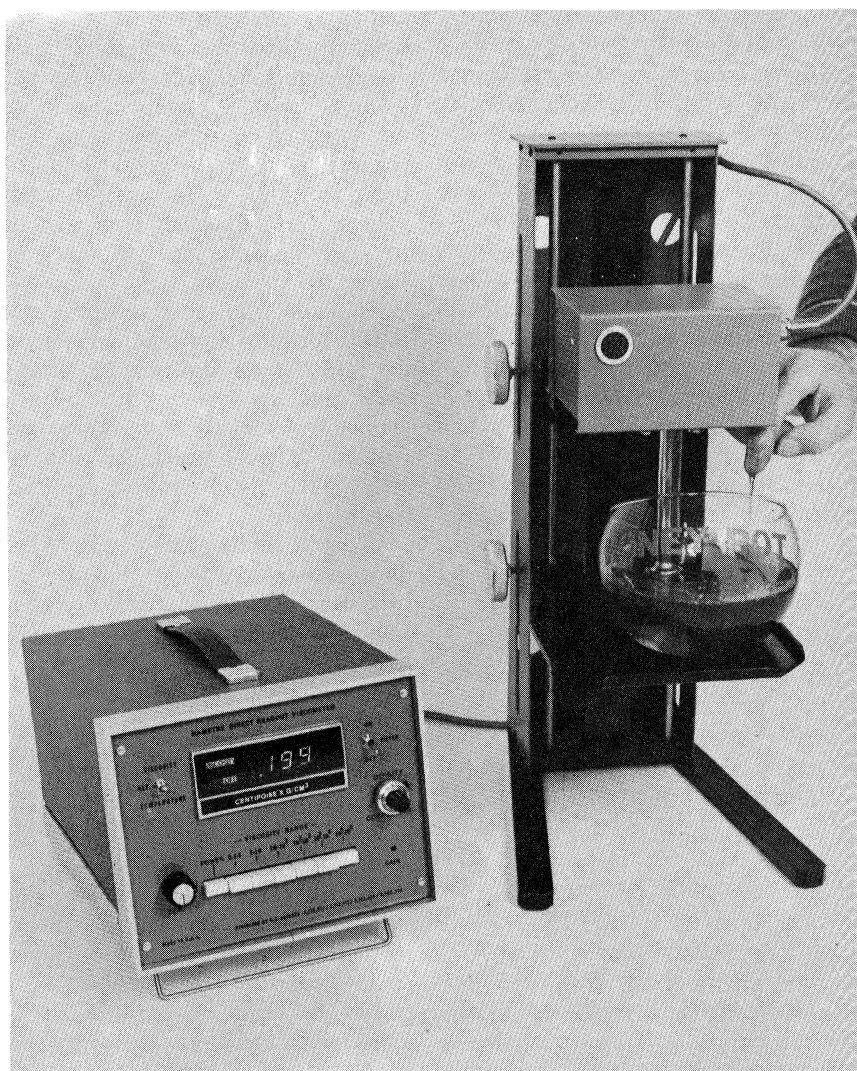
The Model 7-010 viscometer for testing product consistency. (Nametre Corporation, Edison, USA.)
