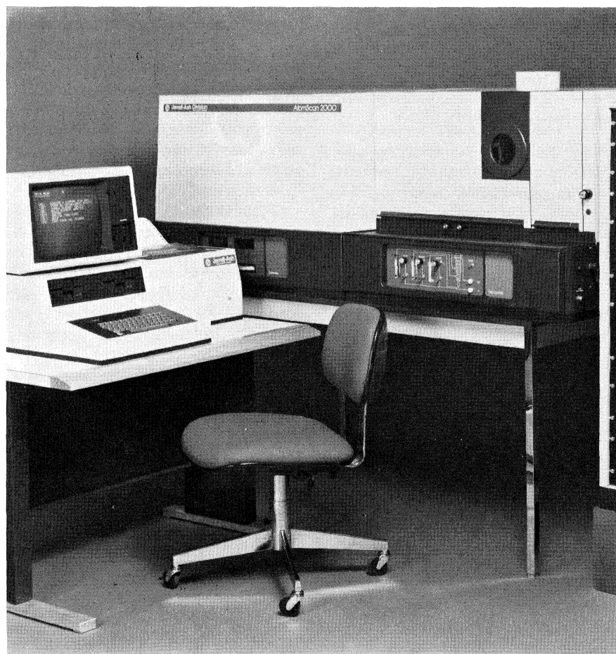
The AtomScan 2000—an ICAP spectrometer for methods development and single- or multi-element analyses. (Jarrell-Ash Division, Fisher Scientific, Waltham, USA.)
