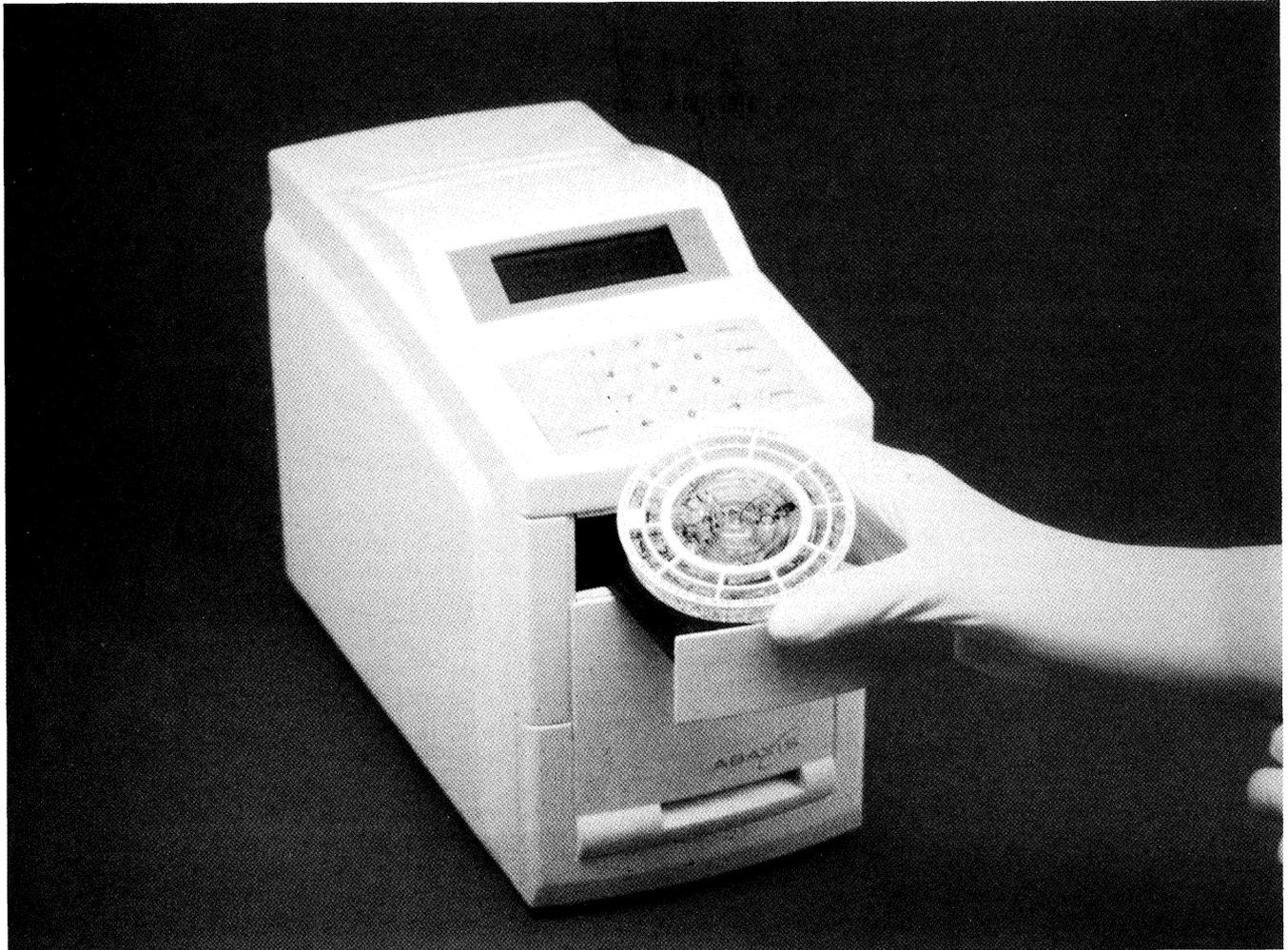
Figure 3. Placing the rotor into the instrument.
