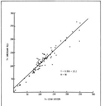
Figure 1. Correlation of  $T_4$  results between manual. (Amersham PEG) and automated (Star system) techniques.
