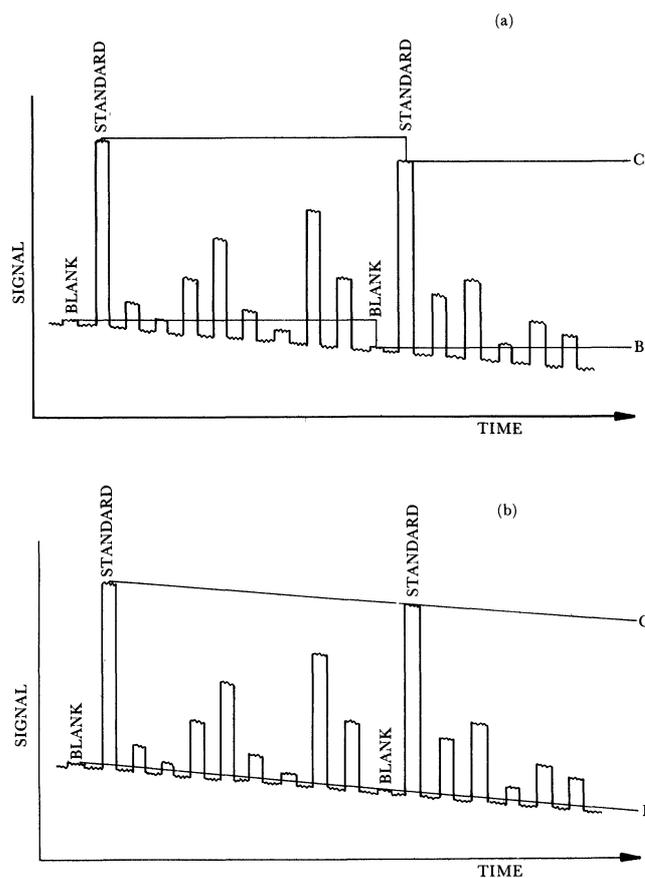
Figure 2. Flame AAS traces indicating assignment of base-line (B) and calibration (C) by an instrument microprocessor (figure 2[a]) and an external microcomputer (figure 2[b]).
