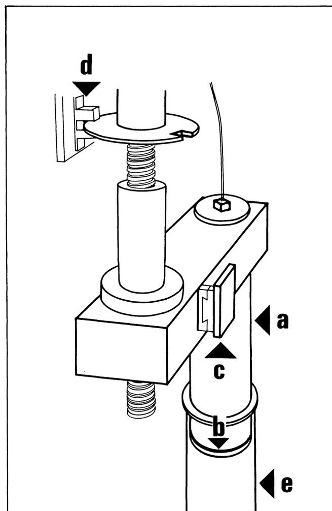
Figure 3. Position sensing and drive mechanism of sampler head.
