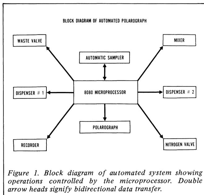
Figure 1. Block diagram of automated system showing operations controlled by the microprocessor. Double arrow heads signify bidirectional data transfer.
