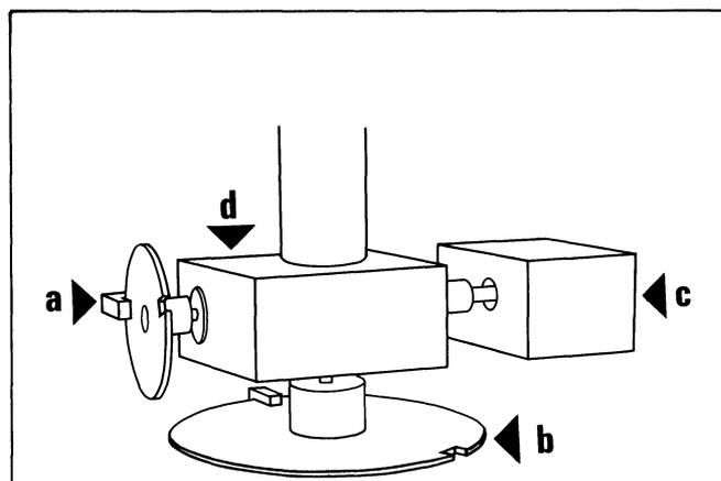
Figure 2. Position sensing and drive mechanism of sample turntable.
