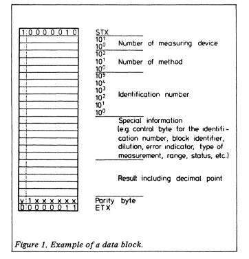
This data block includes the number of the device, the number of the method or test, the sample identification number, some additional information on the status and operation of the measuring instrument, and finally the actual result of the test.
