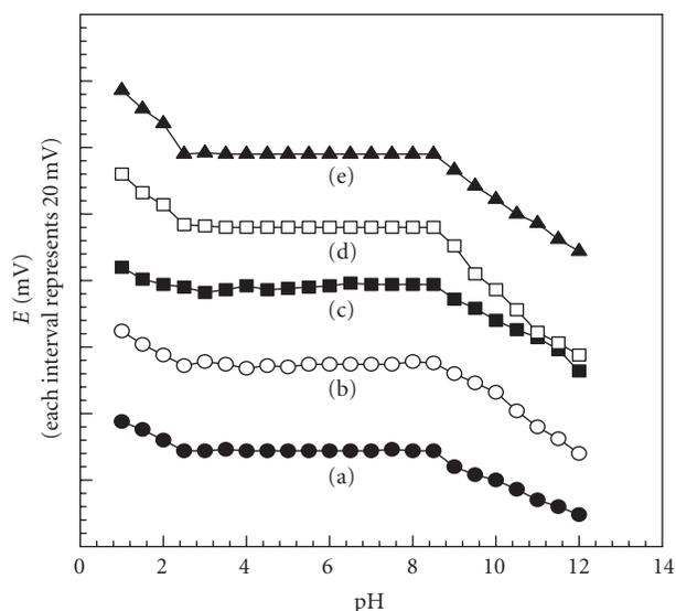
FIGURE 4: Effect of pH of the test solution of concentration  $1 \times 10^{-3}$  M hexoprenaline on the potential response of a-Hx-PTA(I), b-Hx-PTA(II), c-Hx-PTA(III), d-HX-PTA(IV), and e-Hx-PTA(V) electrodes at optimum FIA conditions.
