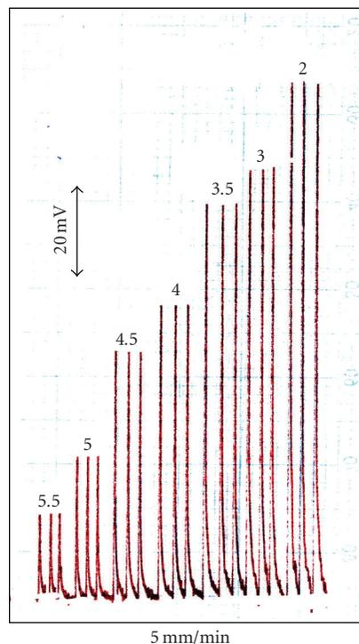
FIGURE 3: Recordings obtained for hexoprenaline solution having  $\text{pHx} = 5.5\text{--}2.0$  using Hx-PTA conventional electrode at optimum FIA conditions.
