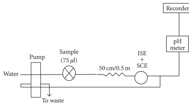
FIGURE 1: Schematic diagram of the flow injection system used in measurements.
