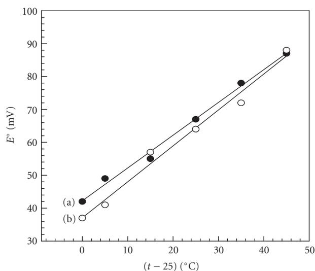
FIGURE 2: Variation of  $E^{\circ}$  of Hx-PTA (a) and Hx-PMA (b) graphite electrodes with temperature.
