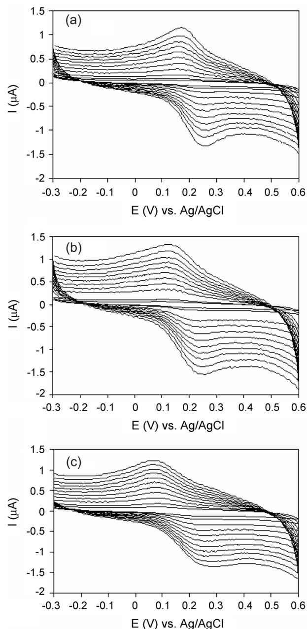
**Figure 4.** Cyclic voltammograms of the gold electrode modified with: (a) Nafion-riboflavin-Hb, (b) Nafion-riboflavin-SOD and (c) Nafion-riboflavin-Cyt *c* in a 50 mM MOPS buffer solution (pH 6.0). Sweep rates (from inner to outer) for (a), (b) and (c) are as follows: 0.025, 0.05, 0.1, 0.2, 0.3, 0.4, 0.5, 0.6, 0.7, 0.8 and 0.9 V s<sup>-1</sup>.
