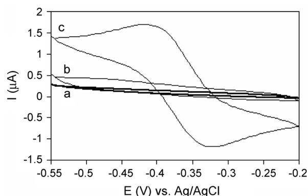
**Figure 1.** Cyclic voltammograms obtained in 50 mM MOPS buffer solution (at pH 6.0) for the (a) gold electrode, (b) Nafion-modified gold electrode and (c) Nafion-riboflavin modified gold electrode at a scan rate of 100 mV/s.
