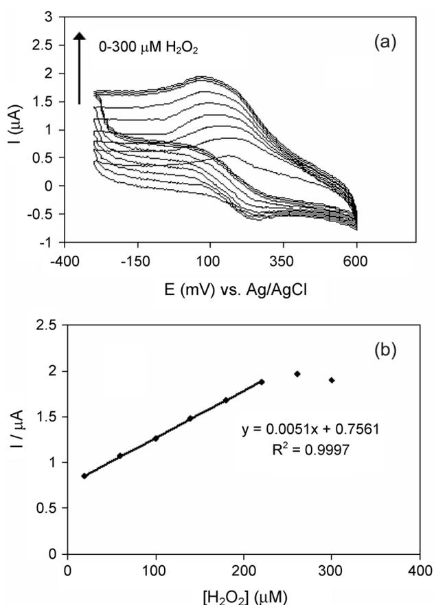
**Figure 5.** (a) Cyclic voltammograms obtained at a Nafion-riboflavin-Hb modified gold electrode for a 50 mM MOPS buffer solution (pH 6) for 0-300 μM concentrations of H<sub>2</sub>O<sub>2</sub> and (b) the relationship between cathodic peak current of hemoglobin and different concentrations of H<sub>2</sub>O<sub>2</sub>.
