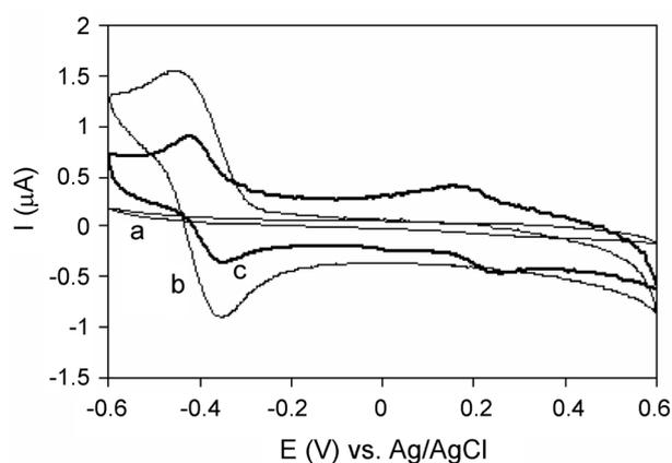
**Figure 3.** Cyclic voltammograms (CVs) obtained in 50 mM MOPS buffer solution at pH 6.0 for (a) Nafion, (b) Nafion-riboflavin and (c) Nafion-riboflavin-protein modified gold electrode at a scan rate of 100 mV/s.
