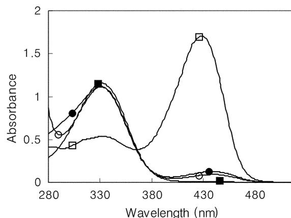
**Figure 1.** The UV-Vis spectra of **1** (■) and **1** in the presence of *n*-butylamine (□), diethylamine (●), and triethylamine (○). [**1**] = 5 × 10<sup>-5</sup> M, [amine] = 5 × 10<sup>-2</sup> M in CHCl<sub>3</sub>.
