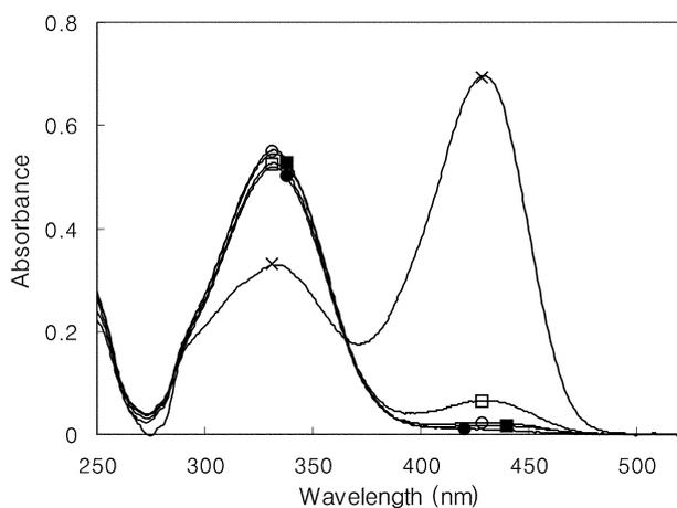
**Figure 2.** UV-Vis absorption spectra of **1** in the absence (■) and presence of *n*-Bu (×), *iso*-Bu (□), *sec*-Bu (○), and *tert*-Bu amines (●) in chloroform.  $[\mathbf{1}] = 2.5 \times 10^{-5} \text{ M}$ .  $[\textit{Butylamine}] = 2.5 \times 10^{-2} \text{ M}$ .
