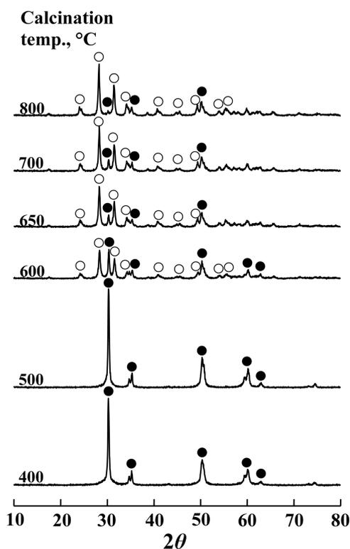
**Figure 3.** X-ray diffraction patterns of 5-CeO<sub>2</sub>-ZrO<sub>2</sub> calcined at different temperatures for 1.5 h: (●), tetragonal phase of ZrO<sub>2</sub>; (○), monoclinic phase of ZrO<sub>2</sub>.
