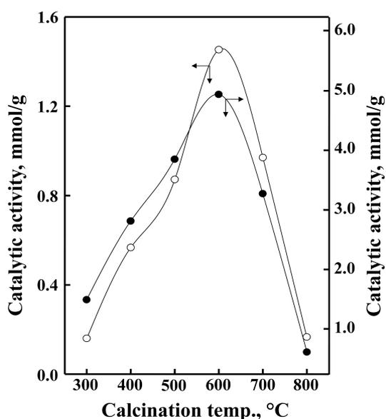
**Figure 9.** Catalytic activities of 10-NiSO<sub>4</sub>/1-CeO<sub>2</sub>-ZrO<sub>2</sub> for 2-propanol dehydration (○) and cumene dealkylation (●) as a function of calcination temperature.
