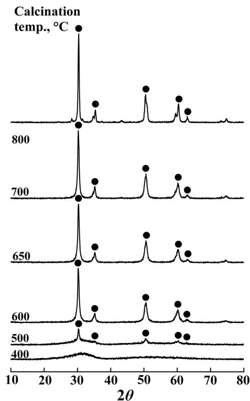
**Figure 4.** X-ray diffraction patterns of 10-NiSO<sub>4</sub>/1-CeO<sub>2</sub>-ZrO<sub>2</sub> as a function of calcination temperature: (●), tetragonal phase of ZrO<sub>2</sub>.
