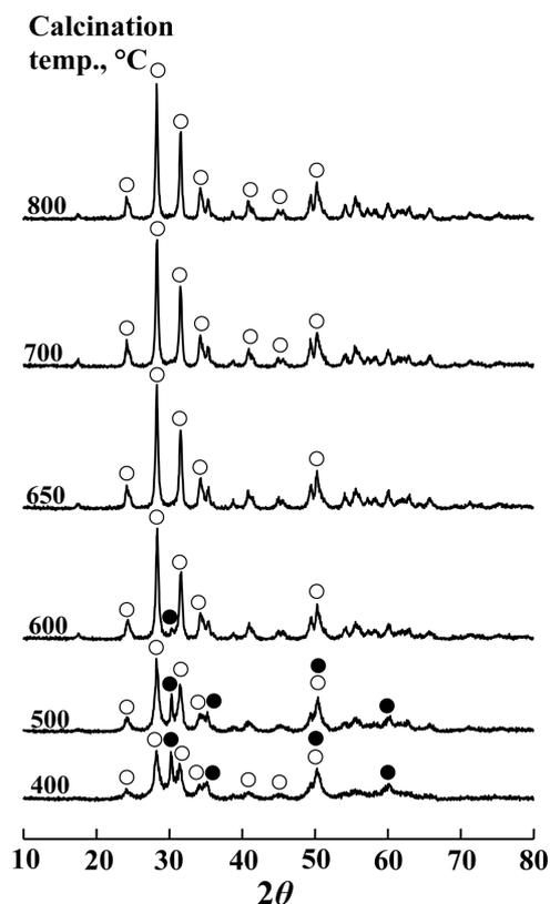
**Figure 2.** X-ray diffraction patterns of 1-CeO<sub>2</sub>-ZrO<sub>2</sub> calcined at different temperatures for 1.5 h: (●), tetragonal phase of ZrO<sub>2</sub>; (○), monoclinic phase of ZrO<sub>2</sub>.
