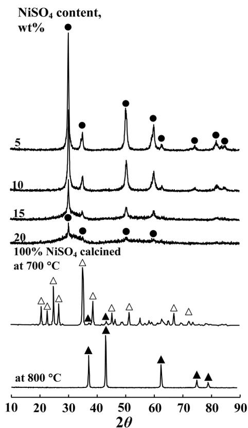
**Figure 6.** X-ray diffraction patterns of NiSO<sub>4</sub>/5-CeO<sub>2</sub>-ZrO<sub>2</sub> having different NiSO<sub>4</sub> contents and calcined 600 °C for 1.5 h: (●), tetragonal phase of ZrO<sub>2</sub>; (△), orthorhombic phase of NiSO<sub>4</sub>; (▲), cubic phase of NiO.
