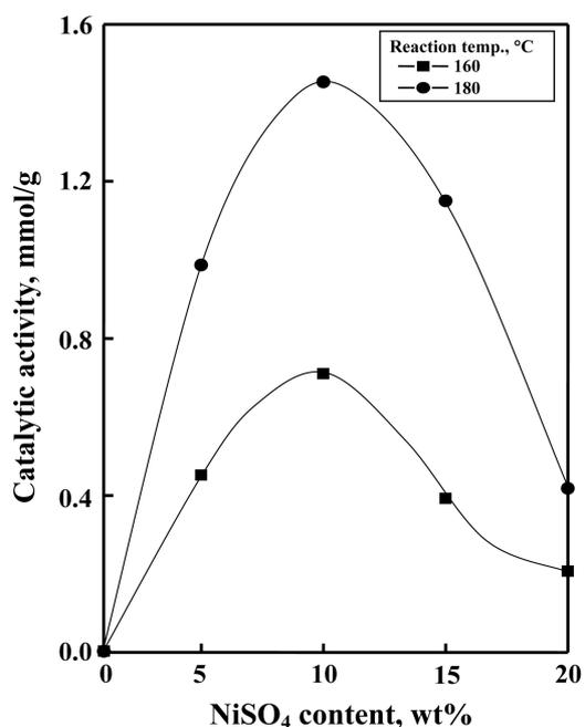
**Figure 10.** Catalytic activities for 2-propanol dehydration as a function of NiSO<sub>4</sub> content.
