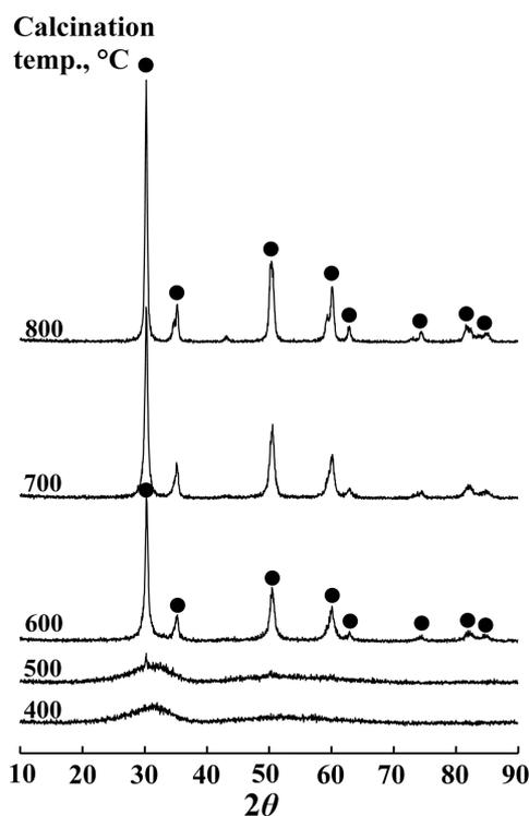
**Figure 5.** X-ray diffraction patterns of 10-NiSO<sub>4</sub>/5-CeO<sub>2</sub>-ZrO<sub>2</sub> as a function of calcination temperature: (●), tetragonal phase of ZrO<sub>2</sub>.
