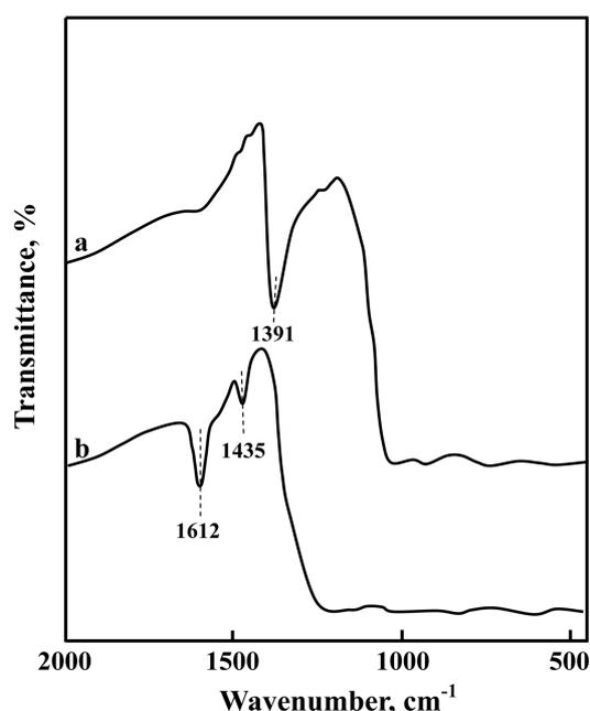
**Figure 8.** Infrared spectra of NH<sub>3</sub> adsorbed on 10-NiSO<sub>4</sub>/1-CeO<sub>2</sub>-ZrO<sub>2</sub>: (a) background of 10-NiSO<sub>4</sub>/1-CeO<sub>2</sub>-ZrO<sub>2</sub> after evacuation at 500 °C for 1 h, (b) NH<sub>3</sub> adsorbed on (a), where gas was evacuated at 230 °C for 1 h.
