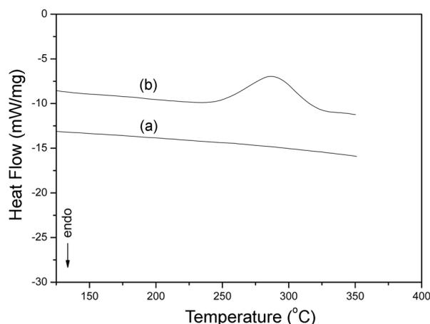
**Figure 4.** DSC curves of (a) PI-CA and (b) PI-DMNB.
