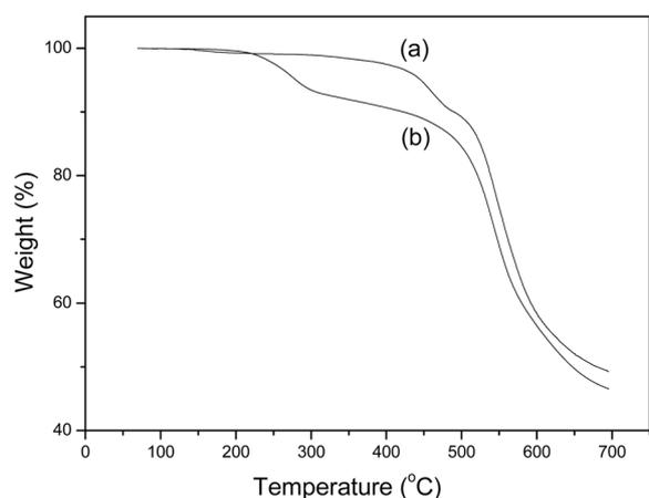
**Figure 3.** TGA curves of (a) PI-CA and (b) PI-DMNB.
