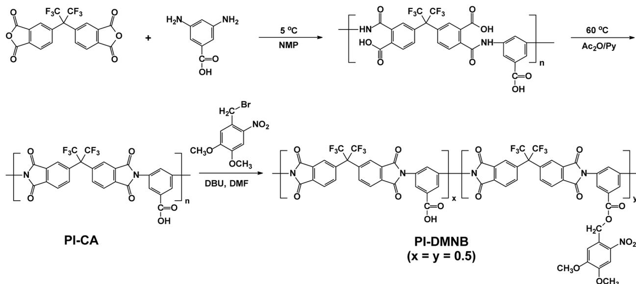
**Scheme 1.** Synthetic diagram of photosensitive polyimide, PI-DMNB.
