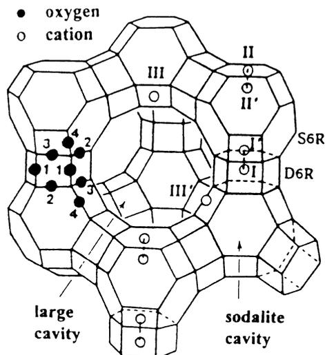
**Figure 1.** Framework structure of zeolite X. Near the center of the each line segment is an oxygen atom. The different oxygen atoms are indicated by the numbers 1 to 4. Silicon and aluminum atoms alternate the tetrahedral intersections, except that Si substitutes for about 4% of the Al's. Extraframework cation positions are labeled with Roman numerals. Site IV, difficult to indicate, is at the center of the supercage.
