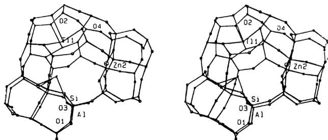
**Figure 5.** A stereoview of a sodalite cavity with two attached D6R in dehydrated  $Zn_{13}Tl_{66}\text{-X}\cdot 2\text{ZnO}$  are shown. One  $Zn^{2+}$  ion at Zn(2) (site I') and three  $Tl^+$  ions at Tl(1) (site I') are shown. About 37.5% of the sodalite cavities may have this arrangement. Ellipsoids of 20% probability are shown.
