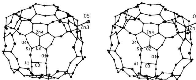
**Figure 3.** A stereoview of the supercage of the dehydrated  $\text{Zn}_{46}\text{-X-8 ZnO}$ . One  $\text{Zn}^{2+}$  ion at Zn(3) (site II'), two  $\text{Zn}^{2+}$  ions at Zn(4) (site II), and one nonframework oxygen O(5) are shown. All of the supercages have this arrangement. Ellipsoids of 20% probability are shown.
