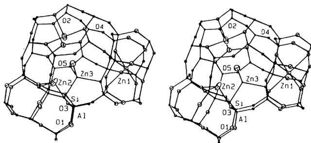
**Figure 2.** A stereoview of a sodalite cavity with two attached D6R in dehydrated  $\text{Zn}_{46}\text{-X-8 ZnO}$ . Shown are one  $\text{Zn}^{2+}$  ion at Zn(1) (site I), three  $\text{Zn}^{2+}$  ions at Zn(2) (site I'), one  $\text{Zn}^{2+}$  ion at Zn(3) (site II'), and one oxygen at O(5) (connected with Zn(3)). About 50% of the sodalite cavities may have this arrangement. Ellipsoids of 20% probability are shown.
