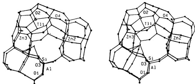
**Figure 4.** A stereoview of a sodalite cavity with two attached D6R in dehydrated  $Zn_{13}Tl_{66}\text{-X}\cdot 2\text{ZnO}$ . Two  $Zn^{2+}$  ions at Zn(2) (site I'), one  $Zn^{2+}$  ion at Zn(3) (site II') and two  $Tl^+$  ions at Tl(1) (site I') are shown. About 25% of the sodalite cavities may have this arrangement. Ellipsoids of 20% probability are shown.
