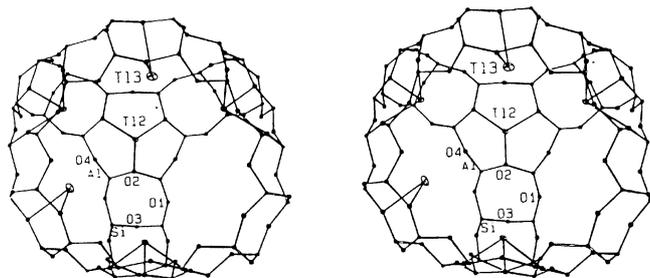
**Figure 7.** A stereoview of the supercage of the dehydrated  $Zn_{13}Tl_{66-X} \cdot 2 ZnO$ . Four  $Tl^+$  ions at Tl(2) (site II) and two  $Tl^+$  ions at Tl(3) (site III') are shown. About 37.5% of the supercages have this arrangement. Ellipsoids of 20% probability are shown.
