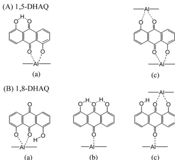
**Figure 2.** Structures of DHAQ in various inorganic matrices.
