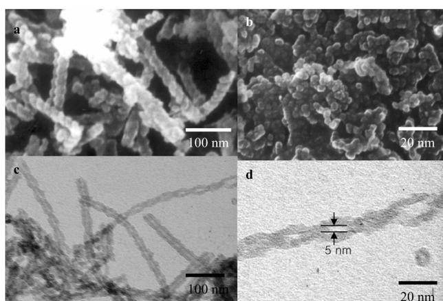
**Figure 2.** FE-SEM image of the silica nanotubes obtained from **1** and **4** [(a) **1** : **4** = 1 : 1 w/w, and (b) **1** : **4** = 9 : 1 w/w.] and (c and e) EF-TEM image of the silica nanotubes obtained from **1**+**4** = 1 : 1 w/w).
