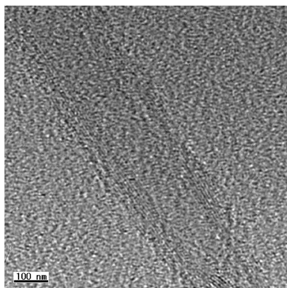
**Figure 4.** HRTEM image of CNT powder produced by decomposition of C<sub>2</sub>H<sub>2</sub> through Pd/Al<sub>2</sub>O<sub>3</sub> at 650 °C, which shows an inside hollow and multiwalled structure.
