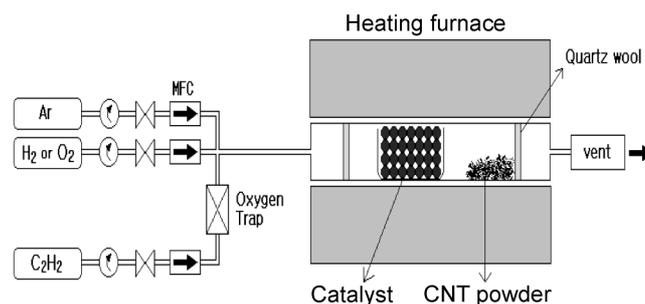
**Figure 1.** Experimental setup used for synthesis of CNTs.
