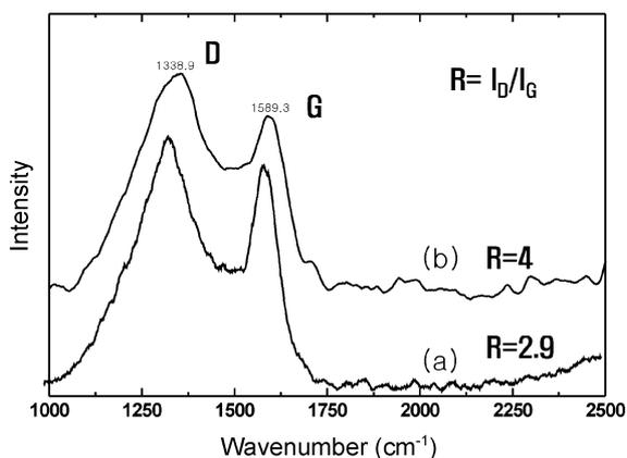
**Figure 5.** Raman spectrum of CNT powder produced by decomposition of C<sub>2</sub>H<sub>2</sub> through Pd/Al<sub>2</sub>O<sub>3</sub> catalyst at (a) 650 °C, (b) 950 °C.
