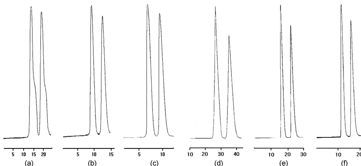
**Figure 2.** Chromatograms of the separation of racemic *N*-acetyl-1-naphthylethylamide (**3**) on preparative CSP 1 at different flow rates (F/R). Mobile phase; 20% 2-propanol in hexane. Sample injection volume (I/V); 0.2 mL (20 mg) (a) column size; 7.8 mm ID  $\times$  250 mm length, F/R 4 mL/min, (b) F/R 6 mL/min, (c) F/R 8 mL/min. (d) column size; 10 mm ID  $\times$  250 mm length, F/R 4 mL/min, (e) F/R 6 mL/min, (f) F/R 8 mL/min.
