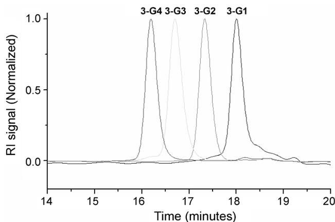
**Figure 3.** GPC diagram of dendrimer **3-Gn**.
