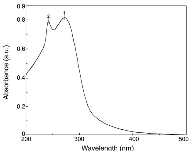
**Figure 2.** UV-visible spectrum of poly(DPSCH) in THF.
